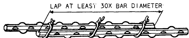
Figure 7-31.-Bars spliced by lapping.
