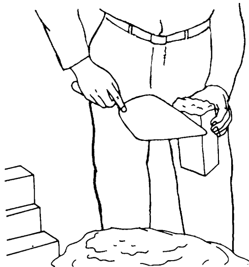
Figure 8-39.-Proper way to hold a brick when buttering the end.
