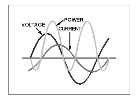
**<u>POWER FACTOR</u>**—The portion of the <u>apparent power</u> dissipated in a circuit is called the power factor of the circuit. It can be expressed as a decimal or a percentage. The formulas for power
