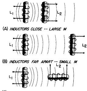
(C) INDUCTOR AXES PERPENDICULAR -- NO M
