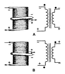
Figure 5-9.—Instantaneous polarity depends on direction of winding.
