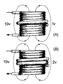
Figure 5-10.—Transformer turns and voltage ratios.
