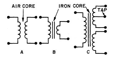
Figure 5-7.—Schematic symbols for various types of transformers.
