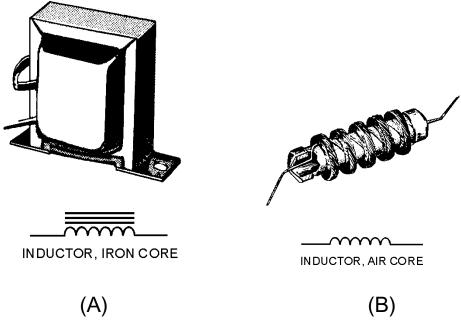
Figure 2-4.—Inductor types and schematic symbols.
