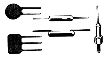
Figure 3-17.—Ceramic capacitors.
