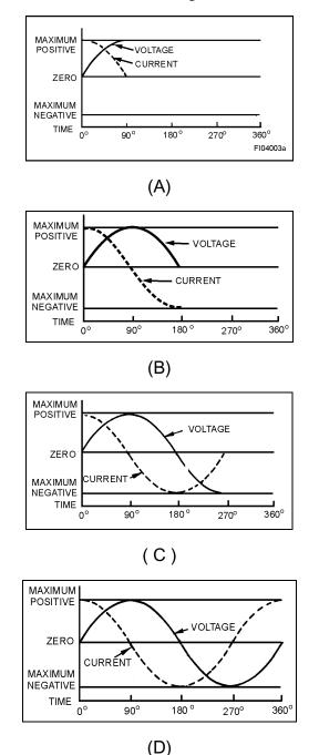
Figure 4-3.—Phase relationship of voltage and current in a capacitive circuit.
