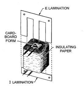
Figure 5-5.—Exploded view of shell-type transformer construction.
