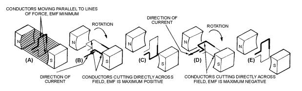
Figure 1-7.—Simple alternating-current generator.
