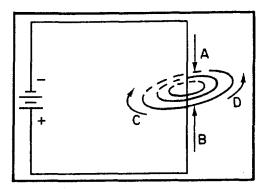
Figure 1B.—A magnetic field surrounding a currentcarrying conductor.
