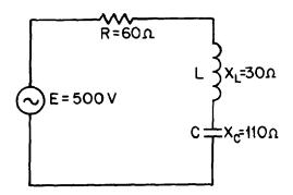
Figure 4-10.—Example circuit for determining power.
