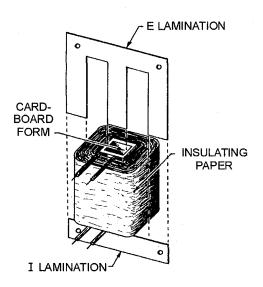
**EXCITING CURRENT**—When voltage is applied to the primary of a transformer, exciting current flows in the primary. The current causes a magnetic field to be set up around both the primary and the secondary windings. The moving flux causes a voltage to be induced into the secondary winding, countering the effects of the counter emf in the primary.
