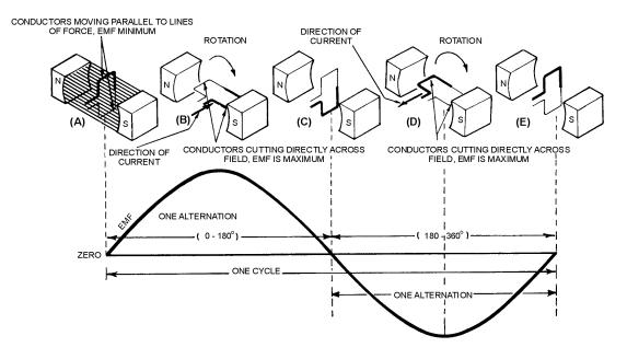
Figure 1-8.—Basic alternating-current generator.
