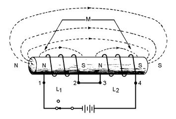
Figure 2-14.—Series inductors with aiding fields.
