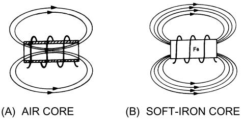
Figure 2-8.—Inductance factor (core material).
