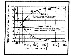
Figure 3E.—Universal time constant chart for RC and RL circuit.
