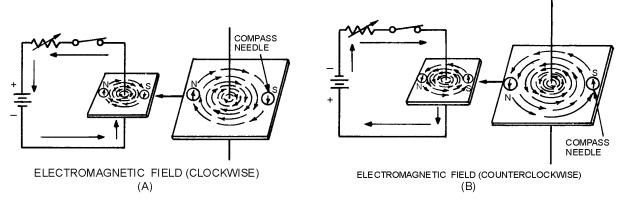
Figure 1-2.—Magnetic field around a current-carrying conductor.
