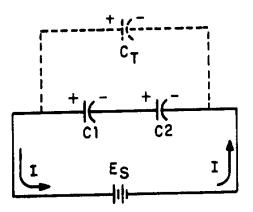
If an electrical circuit contains only two series connected capacitors,  $C_T$  may be computed using the following formula:
