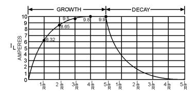
The time constant of an LR circuit may also be defined as the time required for the current in the inductor to grow or decay to its final value if it continued to grow or decay at its initial rate. For all practical purposes, the current in the inductor reaches a maximum value in 5 "Time Constants" and decreases to zero in 5 "Time Constants".
