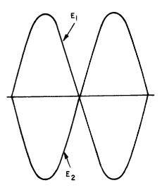
Figure 1-19.—Voltage waves 180° out of phase.
