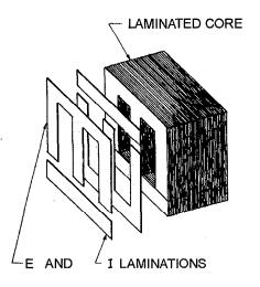
Figure 5-4.—Shell-type core construction.
