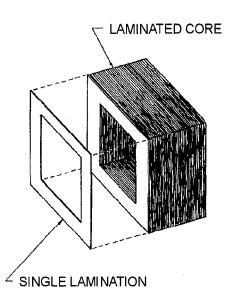
Figure 5-2.—Hollow-core construction.
