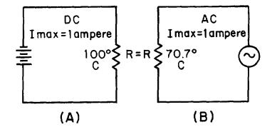
Figure 1-15.—Heating effect of ac and dc.
