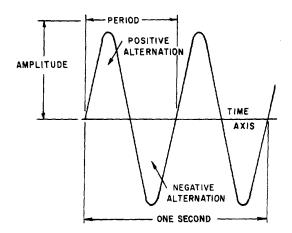
Figure 1-10.—Period of a sine wave.
