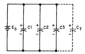
Figure 3-14.—Parallel capacitive circuit.
