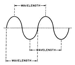
Figure 1-12.—Wavelength measurement.
