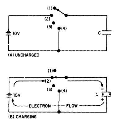
Figure 3-6.—Charging a capacitor.
