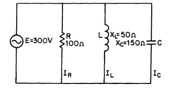
Figure 4-12.—Parallel RLC circuit.
