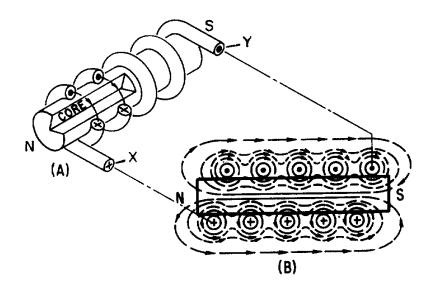
Figure 1-5.—Magnetic field produced by a current-carrying coil.
