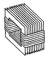
Figure 5-3.—Windings wrapped around laminations.
