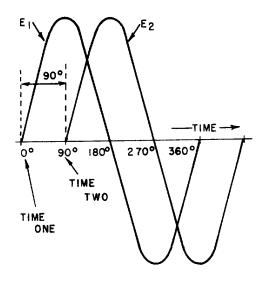
Figure 1-18.—Voltage waves 90° out of phase.
