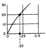
The value selected from the graph means that a capacitor (including the one you are solving for) will reach twenty percent of full charge in twenty-two one hundredths (.22) of one RC time constant. Remember that it takes 100  $\mu$ s for the capacitor to reach 20% of full charge. Since 100  $\mu$ s is equal to .22 RC (twenty-two one-hundredths), then the time required to reach one RC time constant must be equal to:
