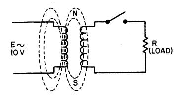
Figure 5-8.—Transformer under no-load conditions.
