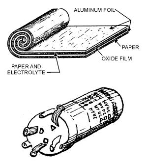
Figure 3-18.—Construction of an electrolytic capacitor.
