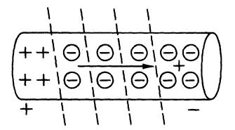
The difference between the charges in the conductor is equal to a difference of potential (or voltage). This voltage caused by the moving magnetic field is called electromotive force (emf).
