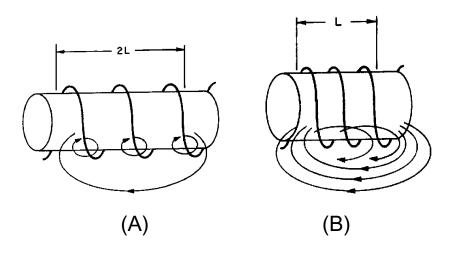
Figure 2-7.—Inductance factor (coil length). CLOSELY WOUND
