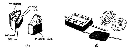
Figure 3-16.—Typical mica capacitors.
