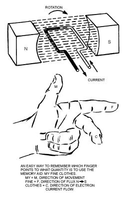
Figure 1-9.—Left-hand rule for generators.
