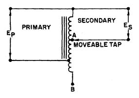
Figure 5-13.—Schematic diagram of an autotransformer.
