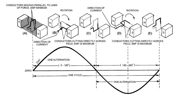
**<u>FREQUENCY</u>**—The number of cycles of ac per second is referred to as the FREQUENCY. AC frequency is measured in hertz. Most ac equipment is rated by frequency as well as by voltage and current.
