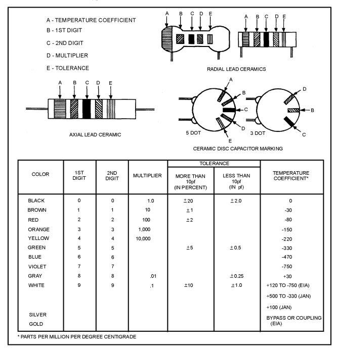
Figure 3-23.—Ceramic capacitor color code.
