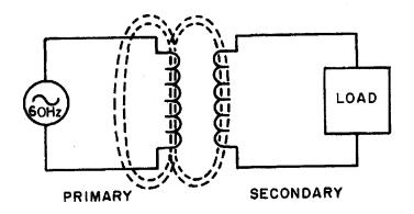
Figure 5-1.—Basic transformer action.
