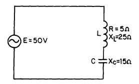
Figure 4-8.—Series LC circuit.
