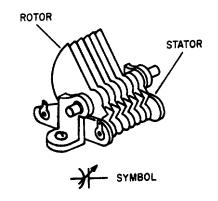
Figure 3-19.—Rotor-stator type variable capacitor.
