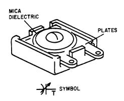
Figure 3-20.—Trimmer capacitor.
