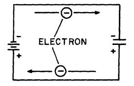
Figure 3-7.—Electron motion during charge.
