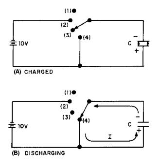
Figure 3-8.—Discharging a capacitor.
