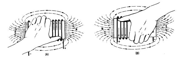
Figure 1-6.—Left-hand rule for coils.
