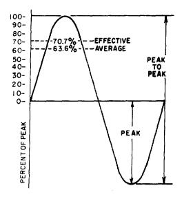
Figure 1-16.—Various values used to indicate sine-wave amplitude.
