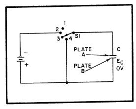
Figure 3C.—Simple capacitor circuit.
