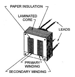
Figure 5-6.—Cutaway view of shell-type core with windings.
