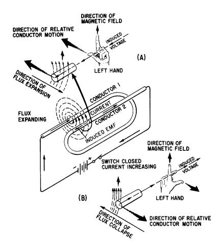
**INDUCTANCE OF A COIL**—The property of inductance can be further increased if the conductor is formed into a coil. Because a coil contains more loops, more of the conductor can be affected by the magnetic field. Inductors (coils) are classified according to core type. The core material is normally either air or soft iron.
