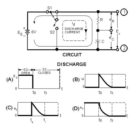
Figure 3-10.—Discharge of an RC Series circuit.
