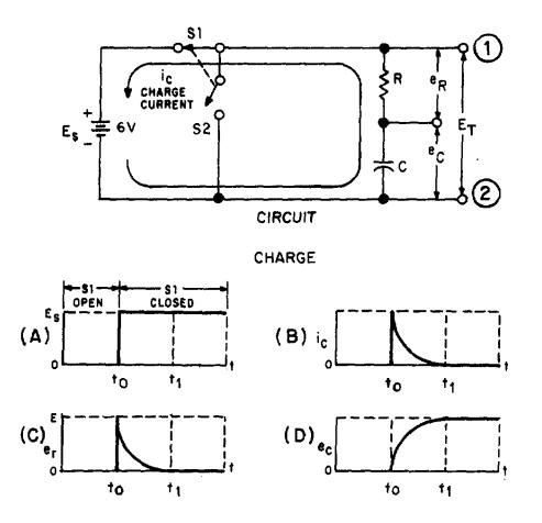
Figure 3-9.—Charge of an RC series circuit.
