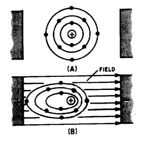
Figure 3-3.—Distortion of electron orbital paths due to electrostatic force.
