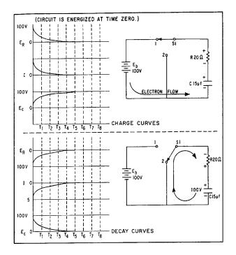
Figure 3D.—RC charge and discharge circuits.
