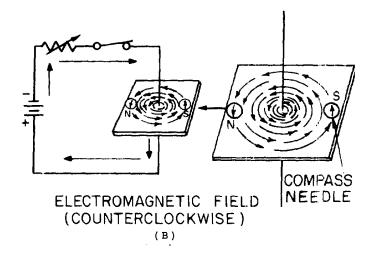
Arrows are generally used in electrical diagrams to indicate the direction of current in a wire. A cross (+) on the end of a cross-sectional view of a wire indicates that current is flowing away from you, while a dot  $(\cdot)$  indicates that current is flowing toward you.
