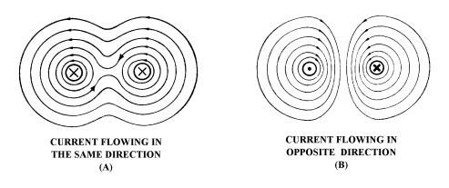
Figure 1-4.—Magnetic field around two parallel conductors.
