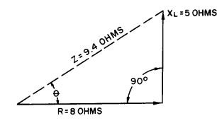
Figure 4-5.—Vector diagram showing relationship of resistance, inductive reactance, and impedance in a series circuit.
