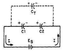
Figure 3-13.—Capacitors in series.
