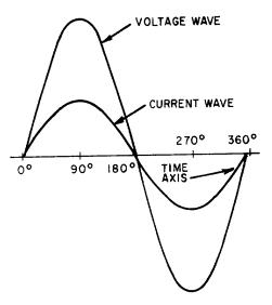
Figure 1-17.—Voltage and current waves in phase.
