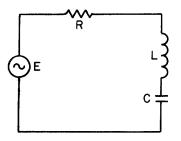
Figure 4-4.—Series RLC circuit.
