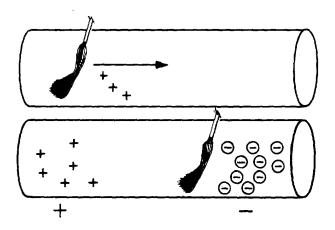
The area from which electrons are moved becomes positively charged, while the area into which electrons are moved becomes negatively charged. The potential difference between these two areas is the electromotive force or emf.
