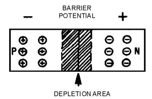
Figure 2-42A.—Pn-junction diode as a variable capacitor.
