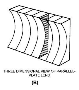
Figure 3-10B.—Waveguide lens.
