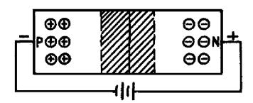
Figure 2-42B.—Pn-junction diode as a variable capacitor.
