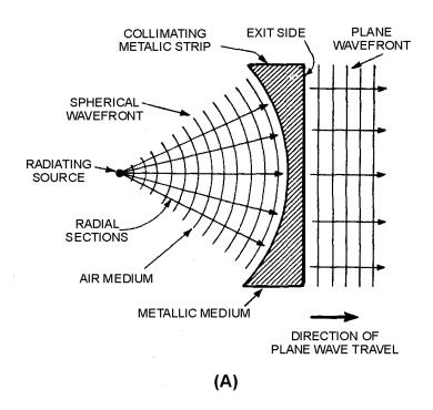
Figure 3-10A.—Waveguide lens.
