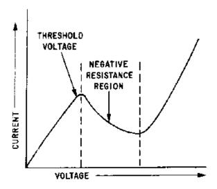
Figure 2-48.—Characteristic curve for a bulk-effect semiconductor.
