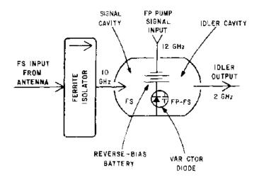
Figure 2-47.—Lower-sideband parametric down-converter.
