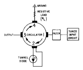
Figure 2-41.—Tunnel-diode amplifier.
