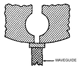
Figure 2-35E.—Magnetron coupling methods.
