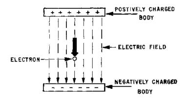
Figure 2-3.—Moving electron losing energy and velocity.
