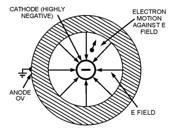
Figure 2-19.—Electron motion in an electric field.
