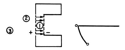
Figure 2-5B.—Buncher cavity action. ELECTRON #1 DECELERATED.
