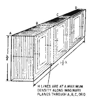
Figure 1-17.—Magnetic field pattern in a waveguide.
