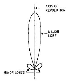
Figure 3-3.—Parabolic radiation pattern.
