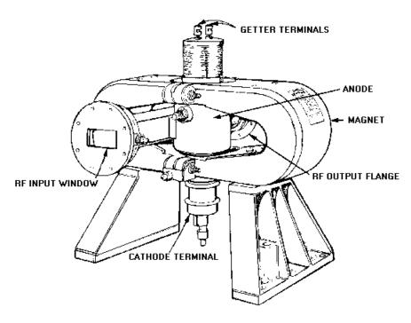
Figure 2-38.—Crossed-field amplifier (Amplitron).
