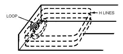
Figure 1-40B.—Loop coupling in a rectangular waveguide.
