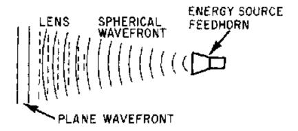
Figure 3-11.—Delay-type lens.
