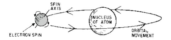
Figure 1-73.—Two types of electron movement.
