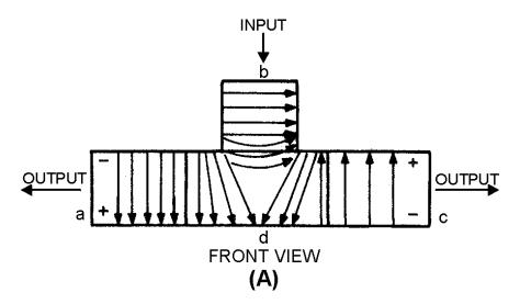
Figure 1-67A.—Magic-T with input to arm b.
