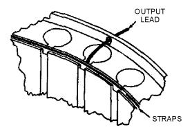
Figure 2-35D.—Magnetron coupling methods.
