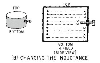
Figure 1-63B.—Methods of changing the resonant frequency of a cavity. CHANGING THE INDUCTANCE.
