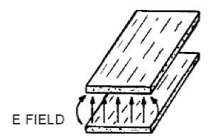
Figure 1-19A.—E field boundary condition. MEETS BOUNDARY CONDITIONS.
