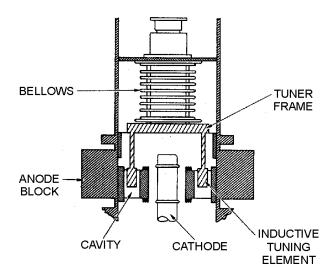
Figure 2-36.—Inductive magnetron tuning.
