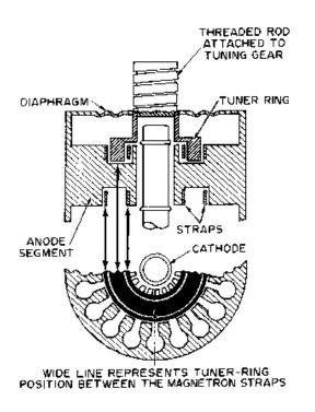
Figure 2-37.—Capacitive magnetron tuning.
