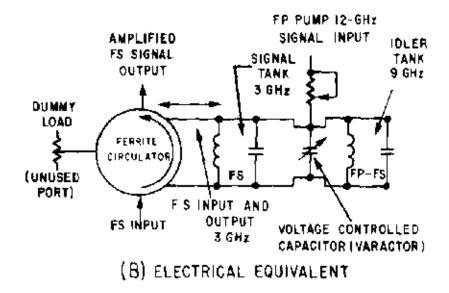
Figure 2-45B.—Nondegenerative parametric amplifier. ELECTRICAL EQUIVALENT.
