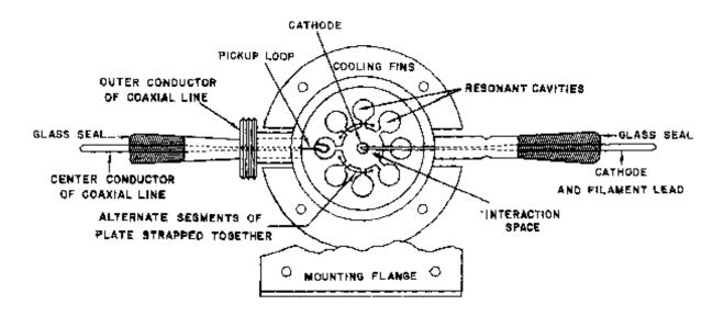
Figure 2-18.—Cutaway view of a magnetron.
