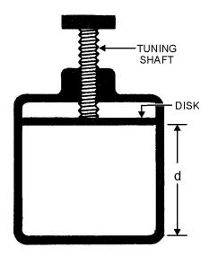
Figure 1-62.—Cavity tuning by volume.
