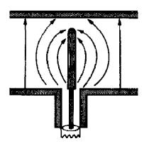
Figure 1-39A.—Probe coupling in a rectangular waveguide.
