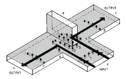
Figure 1-68.—Magic-T with input to arm d.
