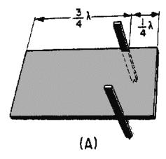
Figure 1-34A.—Waveguide operation in other than dominant mode.
