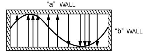
Figure 1-30.—Full-sine E field distribution.
