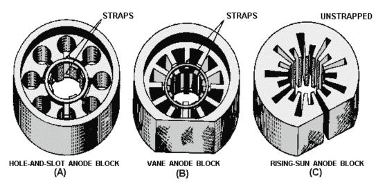
Figure 2-27.—Common types of anode blocks.
