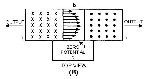
Figure 1-67B.—Magic-T with input to arm b.
