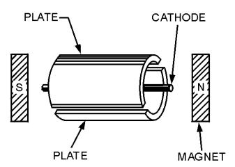
Figure 2-23A.—Split-anode magnetron.
