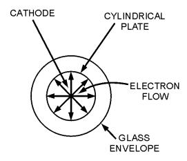
Figure 2-21B.—Basic magnetron. END VIEW OMITTING MAGNETS.
