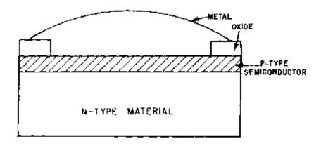
Figure 2-52.—Schottky-barrier diode.
