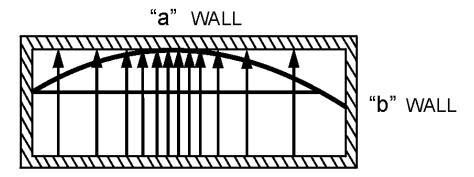
Figure 1-29.—Half-sine E field distribution.
