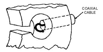
Figure 2-35A.—Magnetron coupling methods.
