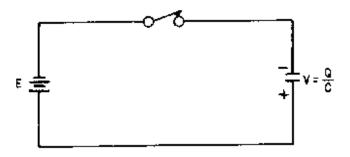
Figure 2-43.—Voltage amplification from a varying capacitor.
