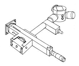
Figure 2-46.—Parametric amplifier.
