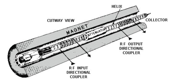
Figure 2-13.—Physical construction of a twt.
