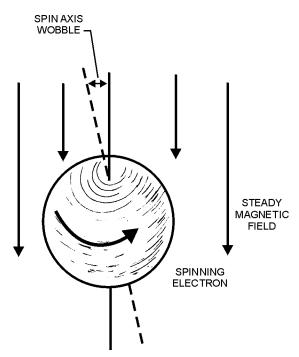
Figure 1-74.—Electron wobble in a magnetic field.
