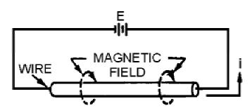
Figure 1-14.—Magnetic field on a single wire.
