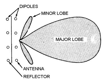
Figure 3-13.—Field pattern of an antenna array.
