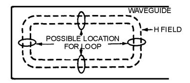
Figure 1-40C.—Loop coupling in a rectangular waveguide.
