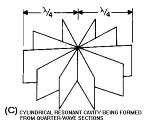
Figure 1-59C.—Development of a cylindrical resonant cavity. CYLINDRICAL RESONANT CAVITY BEING FORMED FROM QUARTER-WAVE SECTIONS.
