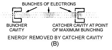
Figure 2-6B.—Removing energy from a velocity-modulated beam.
