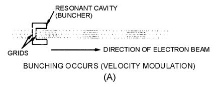
Figure 2-6A.—Removing energy from a velocity-modulated beam.
