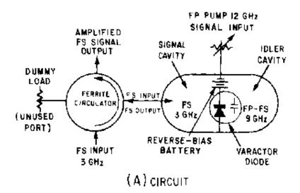
Figure 2-45A.—Nondegenerative parametric amplifier. CIRCUIT.
