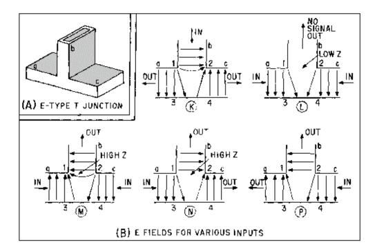
Figure 1-64.—E fields in an E-type T junction.
