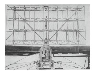
Figure 3-15.—Bedspring array.
