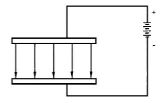
Figure 1-11A.—Simple electric fields. CAPACITOR.
