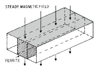
Figure 1-72.—Ferrite attenuator.
