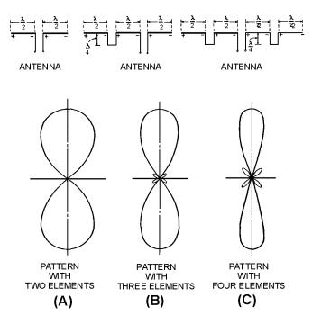
Figure 3-14.—Horizontal array field patterns.
