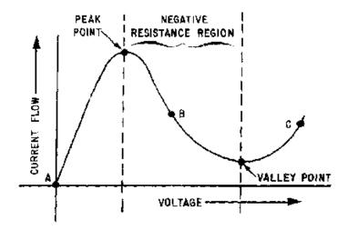
Figure 2-39.—Tunnel-diode characteristic curve.
