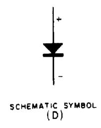
Figure 2-51D.—Point-contact diode. SCHEMATIC SYMBOL.
