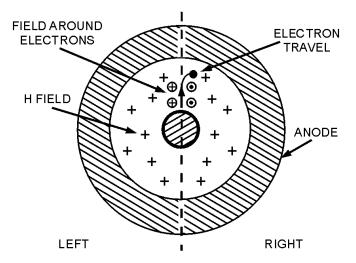
Figure 2-20.—Electron motion in a magnetic field.
