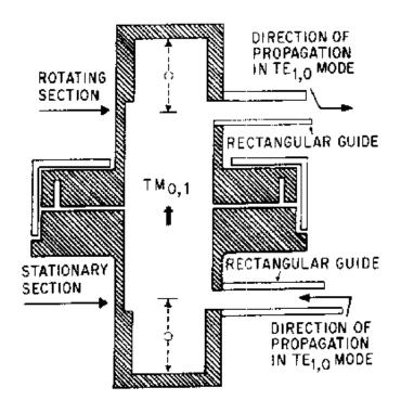
Figure 1-52.—Rotating joint.
