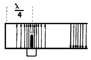
Figure 1-39B.—Probe coupling in a rectangular waveguide.
