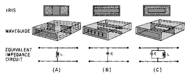
Figure 1-42.—Waveguide irises.
