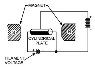
Figure 2-21A.—Basic magnetron. SIDE VIEW.
