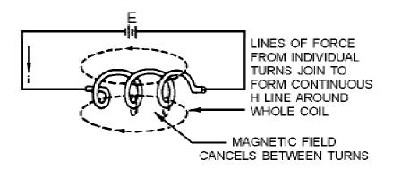
Figure 1-15.—Magnetic field on a coil.
