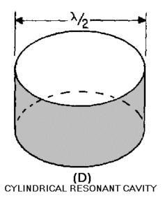
Figure 1-59D.—Development of a cylindrical resonant cavity. CYLINDRICAL RESONANT CAVITY.
