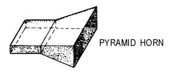
Figure 1-44C.—Waveguide horns. PYRAMID HORN.
