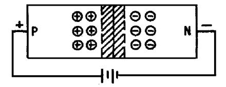
Figure 2-42C.—Pn-junction diode as a variable capacitor.
