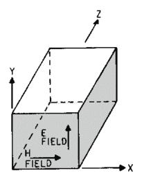
Figure 1-61.—Rectangular cavity resonator.
