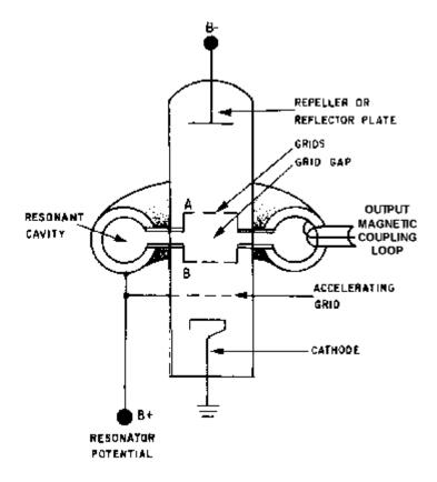
Figure 2-9.—Functional diagram of a reflex klystron.
