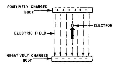
Figure 2-2.—Moving electron gaining velocity and energy.
