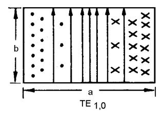
Figure 1-36.—Dominant mode in a rectangular waveguide.
