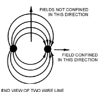
Figure 1-1.—Fields confined in two directions only.
