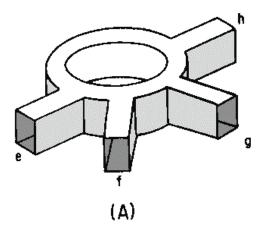
Figure 1-71A.—Hybrid ring with wavelength measurements.
