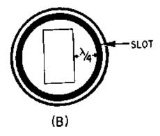
Figure 1-51B.—Choke joint.
