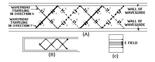
The **MODES** in waveguides are divided into two categories: (1) the TRANSVERSE ELECTRIC (TE) mode and (2) the TRANSVERSE MAGNETIC (TM) mode. Subscripts are used to complete the
