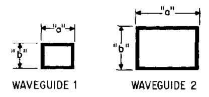
Figure 1-9.—Labeling waveguide dimensions.
