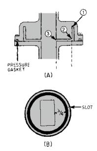
**DIRECTIONAL COUPLERS** are devices that permit the sampling of the energy in a waveguide. Directional couplers may be constructed to sample energy in one direction only or in both directions. The energy removed by the directional coupler is a small sample that is proportional to the magnitude of the energy in the waveguide. An example of a directional coupler is shown in the illustration.
