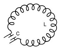
Figure 2-29B.—Equivalent circuit of a hole-and-slot cavity.
