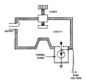
Figure 2-40.—Tunnel-diode oscillator.
