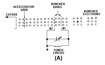
Figure 2-4A.—Electron gun with buncher grids.
