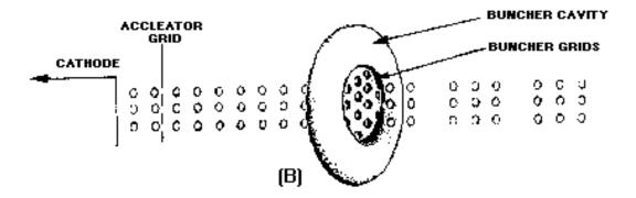
Figure 2-4B.—Electron gun with buncher grids.
