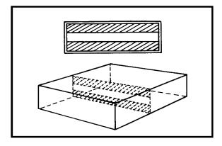
Figure 1B.—Waveguide iris.
