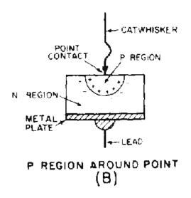
Figure 2-51B.—Point-contact diode. P REGION AROUND POINT.
