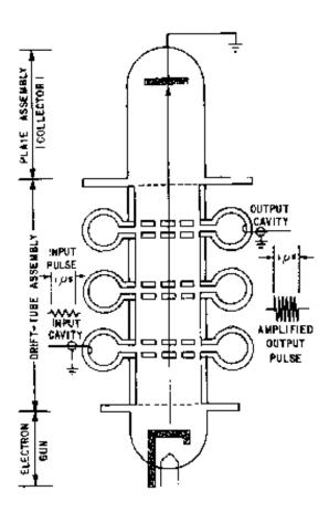
Figure 2-8.—Three-cavity klystron.
