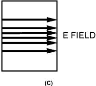
Figure 1-25.—Wavefronts in a waveguide.
