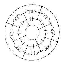
Figure 2-31.—Cavities in parallel because of strapping.
