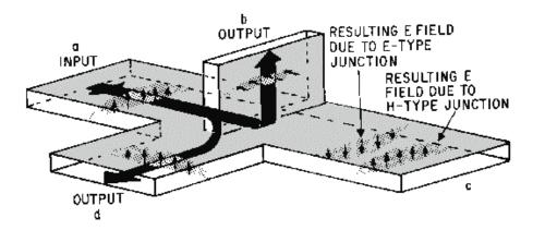
Figure 1-69.—Magic-T with input to arm a.
