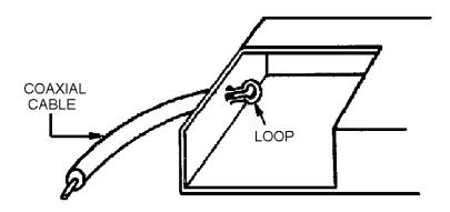
Figure 1-40A.—Loop coupling in a rectangular waveguide.
