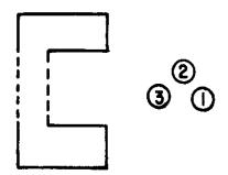
Figure 2-5E.—Buncher cavity action. ELECTRONS BEGINNING TO BUNCH, DUE TO VELOCITY DIFFERENCES.
