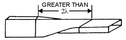
Figure 1-49.—Waveguide twist.
