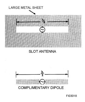
Figure 3-18.—Slot antenna and complementary dipole.
