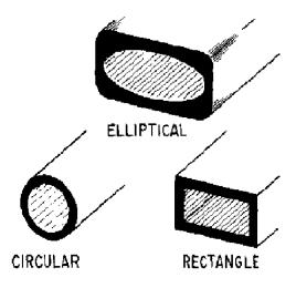
Figure 1-3.—Waveguide shapes.
