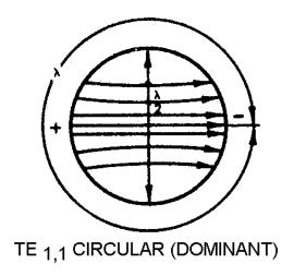
Figure 1-37.—Counting wavelengths in a circular waveguide.
