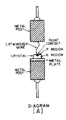
Figure 2-51A.—Point-contact diode. DIAGRAM.
