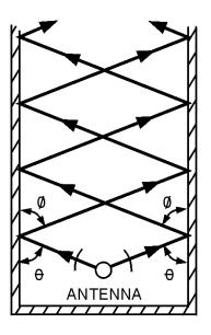
Figure 1-27B.—Different frequencies in a waveguide.
