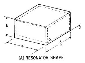
Figure 1-58A.—Rectangular waveguide cavity resonator. RESONATOR SHAPE.
