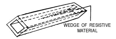
Figure 1-45C.—Terminating waveguides.
