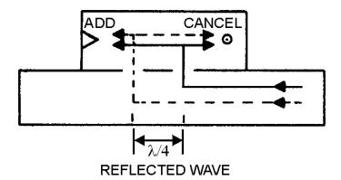
Figure 1-55.—Reflected wave in a directional coupler.
