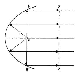
Figure 3-2.—Parabolic reflector radiation.
