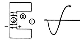
Figure 2-5D.—Buncher cavity action. ELECTRON #3 ACCELERATED.
