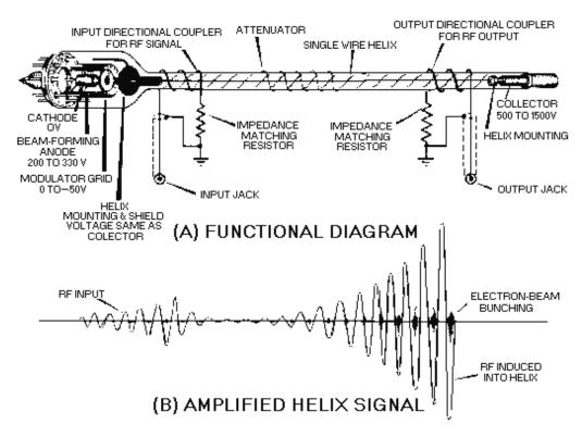
Figure 2-15.—Functional diagram of a twt.
