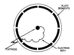
Figure 2-26.—Electron path in an electron-resonance magnetron.
