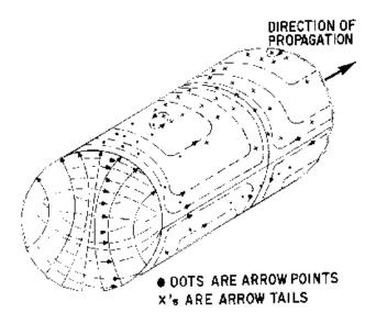
Figure 1-35.—Dominant mode in a circular waveguide.
