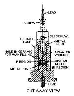
Figure 2-51C.—Point-contact diode. CUT AWAY VIEW.
