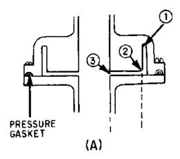
Figure 1-51A.—Choke joint.
