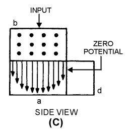
Figure 1-67C.—Magic-T with input to arm b.
