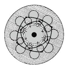
Figure 2-34.—Alternate segments connected by strapping rings.
