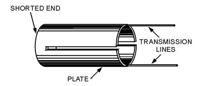
Figure 2-25.—Plate tank circuit of a magnetron.
