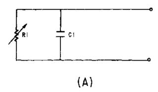
Figure 2-53A.—Diode equivalent circuit (pin).
