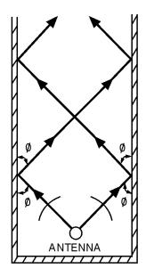
Figure 1-27A.—Different frequencies in a waveguide.
