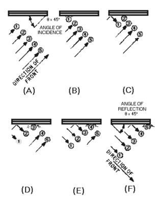
Figure 1-26.—Reflection of a single wavefront.
