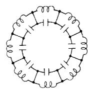
Figure 2-30.—Cavities connected in series.
