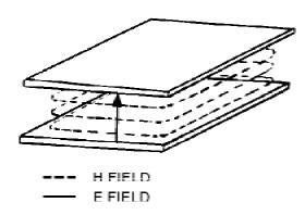
Figure 1-20.—H field boundary condition.
