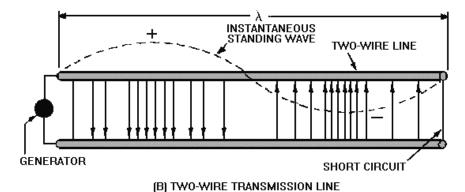
Figure 1-11B—Simple electric fields. TWO-WIRE TRANSMISSION LINE.
