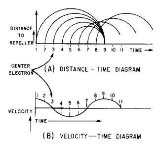
Figure 2-10.—Electron bunching diagram.
