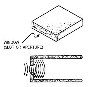
Figure 1-41.—Slot coupling in a waveguide.
