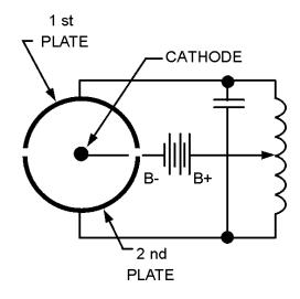
Figure 2-23B.—Split-anode magnetron.
