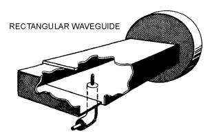
Figure 1-39C.—Probe coupling in a rectangular waveguide.
