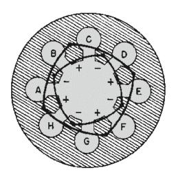
Figure 2-28.—Strapping alternate segments.
