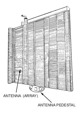
Figure 3-16.—Frequency-sensitive antenna.
