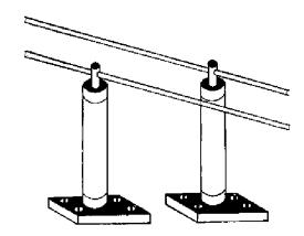
Figure 1-5.—Two-wire transmission line using ordinary insulators.
