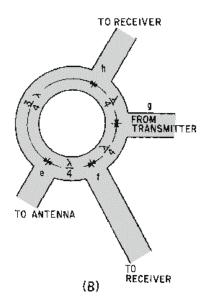
Figure 1-71B.—Hybrid ring with wavelength measurements.
