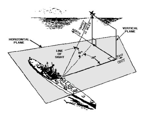
Figure 3-1.—Radar target position.
