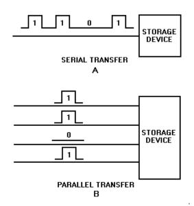
Figure 3-29. —Data transfer methods: A. Serial transfer; B. Parallel transfer.
