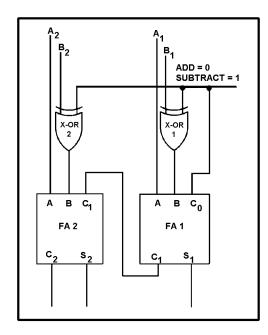
Figure 4D.—Adder/subtracter circuit.
