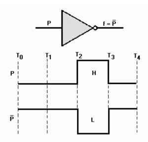
Figure 2-10. —Inverter input and resultant output.
