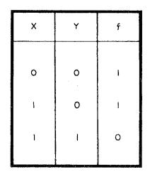
Figure 3D. —Incomplete NAND gate Truth Table.
