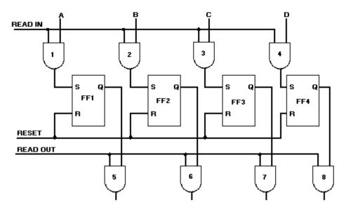
Figure 3-28. —Four-bit parallel register.
