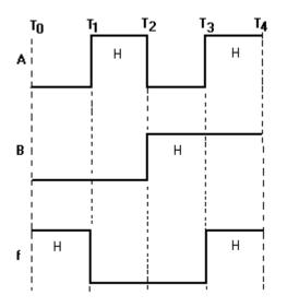
Figure 3-5. —Exclusive NOR gate timing diagram.
