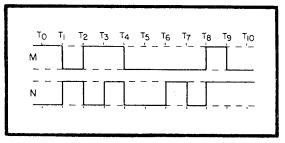
Figure 3E. —Input signal timing diagram.
