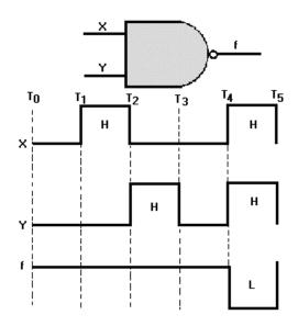
Figure 2-13. —NAND gate input and output signals.
