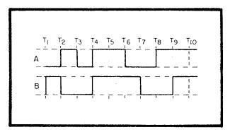
Figure 3A.—AND gate timing diagram.
