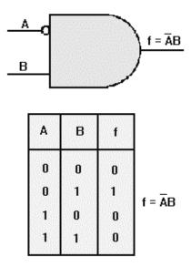
Figure 2-17. —AND gate with one inverted input.
