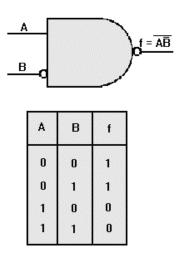
Figure 2-19. —NAND gate with one inverted input.
