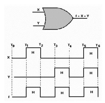
Figure 2-8. —OR gate input and output signals.
