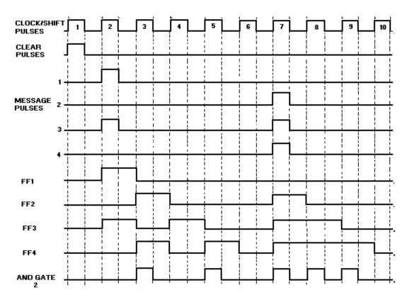
Figure 3-32. —Parallel-to-serial conversion timing diagram.
