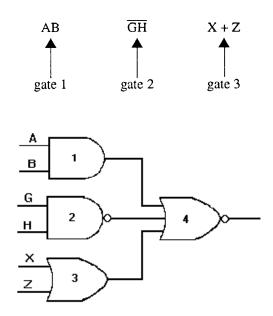
Figure 2-25. —Logic gate combinations.
