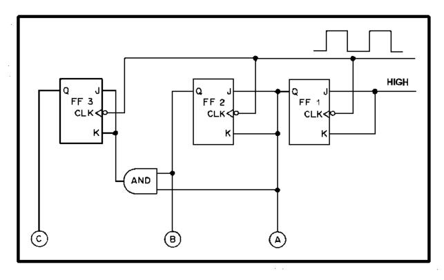
Figure 4H.—Counter circuit.
