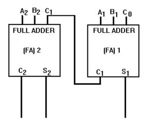
Figure 3-9. —Parallel binary adder.
