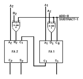
Figure 3-11. — R's complement adder/subtracter.
