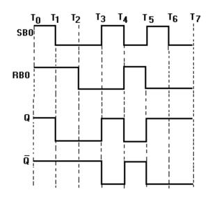
Figure 3-13. —R-S flip-flop with inverted inputs timing diagram.
