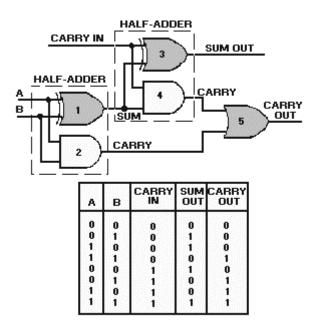
Figure 3-8. —Full adder and Truth Table.
