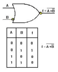
Figure 2-22. —NOR gate with one inverted input.
