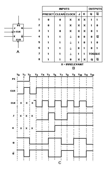
Figure 3-18. —J-K flip-flop: A. Standard symbol; B. Truth Table; C. Timing diagram.
