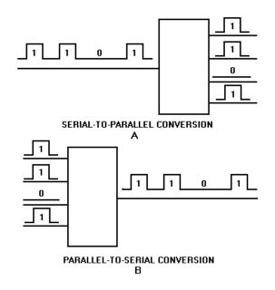
Figure 3-30. —Data conversion methods: A. Serial-to-parallel; B. Parallel-to-serial.
