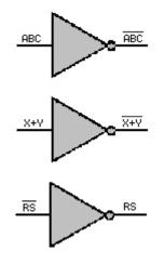
The vinculum, or NOT sign, is placed over the entire output or removed from the output, depending on the input. If we applied  $A\overline{B}C$  to an inverter, the output would be  $\overline{A\overline{B}C}$ . And if we ran that output through another inverter, the output would be  $A\overline{B}C$
