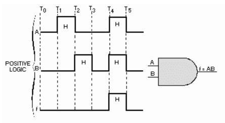
Figure 2-4. —AND gate input and output signals.
