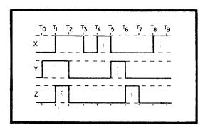
Figure 3C. — OR gate timing diagram.
