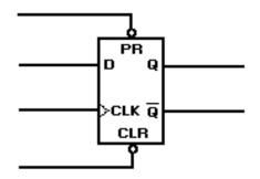
Figure 3-17. —D flip-flop with PR and CLR inputs.
