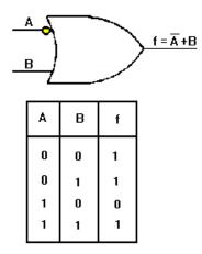
Figure 2-20. —OR gate with one inverted input.
