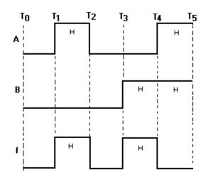
Figure 3-3. —Exclusive OR gate timing diagram.
