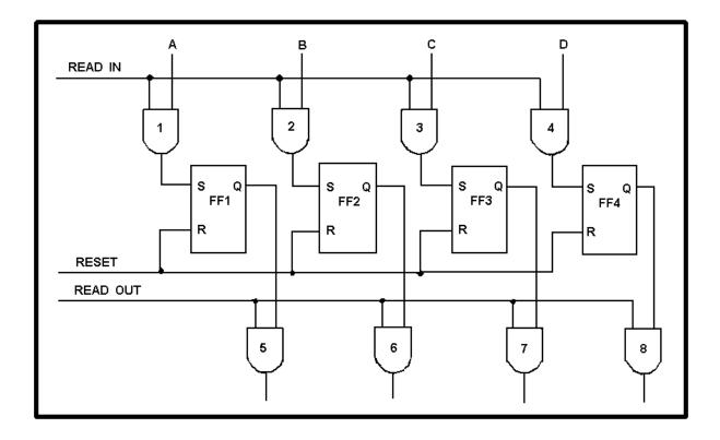
Figure 4L.—Parallel register.
