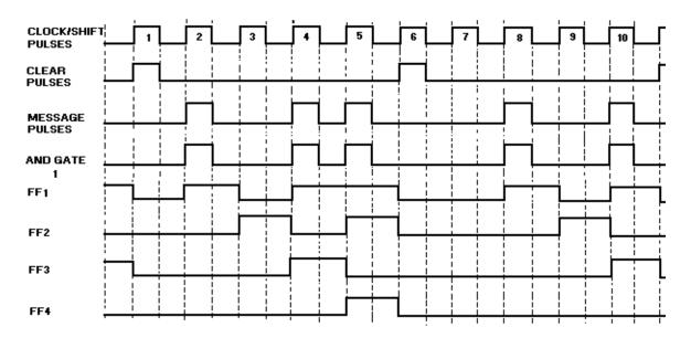
Figure 3-33. —Serial-to-parallel conversion timing diagram.
