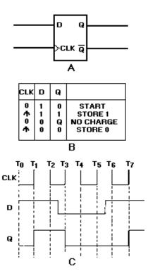
Figure 3-16. — D flip-flop: A. Standard symbol; B. Truth Table; C. Timing diagram.
