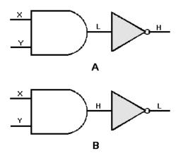
Figure 2-12. —NAND gate equivalent circuit: A. Either X or Y or both are LOW; B. Both X and Y are HIGH.
