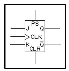
Figure 4F.—Standard symbol for a J-K flip-flop.
