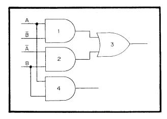
Figure 4B.—Logic circuit.
