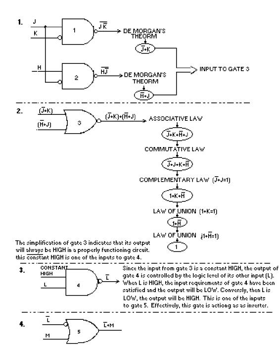
Figure 2-27. —Logic circuit simplification process.
