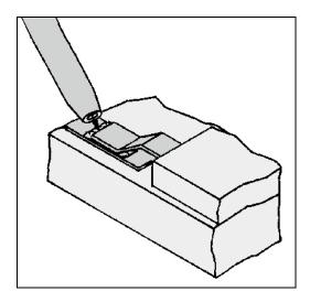
Figure 3-2.—Hot air jet conformal coating removal.
