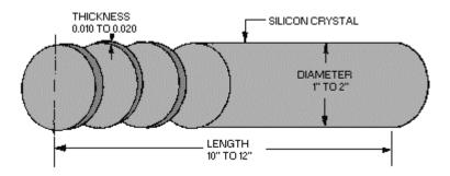
Figure 1-10.—Silicon crystal and wafers.
