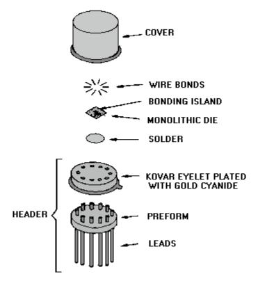
Figure 1-19.—Exploded TO-5.
