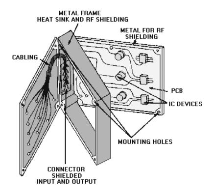
Figure 1-44.—Ground planes and shielding.
