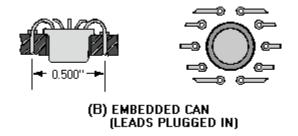
Figure 1-21B.—TO-5 mounting EMBEDDED CAN(LEADS PLUGGED IN)
