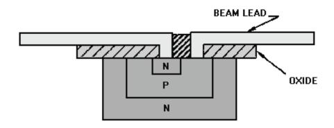
Figure 1-27.—Beam-lead technique.
