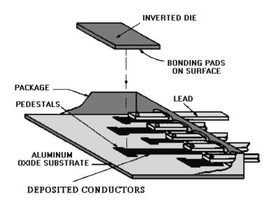
Figure 1-26.—Flip-chip package.
