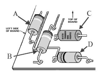
Figure 2A.—Component mounting.
