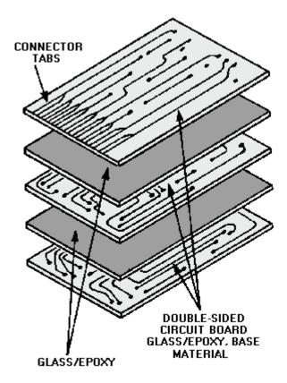
Figure 1-39.—Multilayer pcb.
