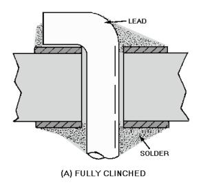
Component **LEADS** are terminated either through the board, above the board, or on the board.
