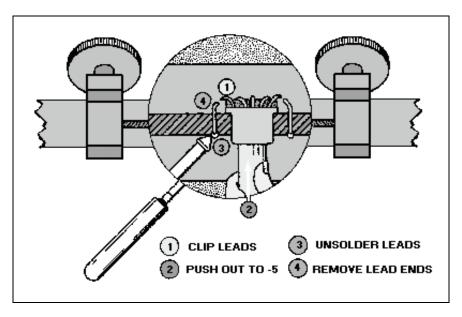
Figure 3-20.—Imbedded TO removal.
