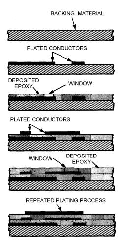
Figure 1-42.—Layer build-up technique.
