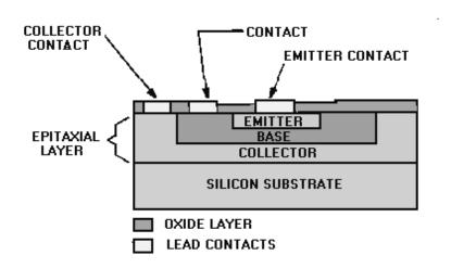
Figure 1-13.—Planar-epitaxial transistor.
