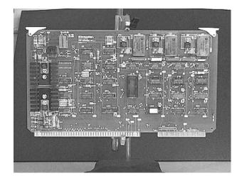
A MICROCIRCUIT MODULE is an assembly of microcircuits or a combination of microcircuits and discrete components packaged as a replaceable unit.
