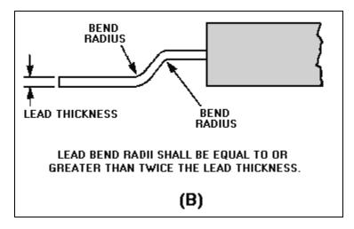
Figure 3-22B.—Properly formed flat pack leads.
