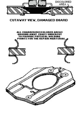
Figure 3-29.—Repair of burned boards.
