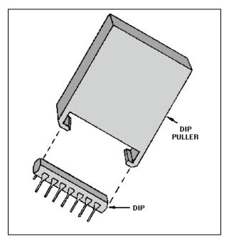
Figure 3-18.—Typical DIP puller.
