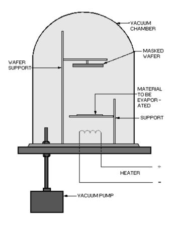
Figure 1-14.—Vacuum evaporation oven.
