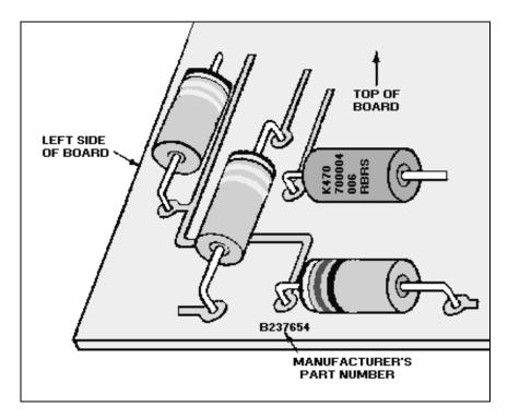
Figure 3-15.—Component arrangement.
