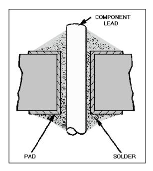
Figure 3-6.—Straight-through termination.
