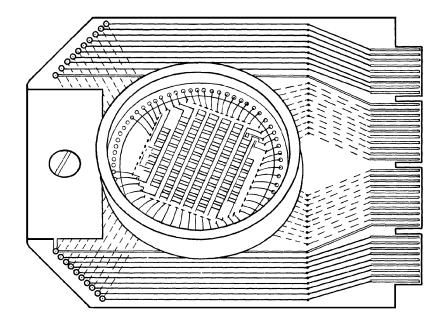
Figure 1-6.—Large-scale integration device (lsi).
