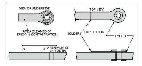
Figure 3-25.—Replacement of damaged termination pad.
