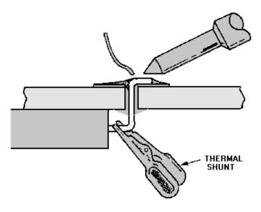
Figure 3-16.—Thermal shunt.
