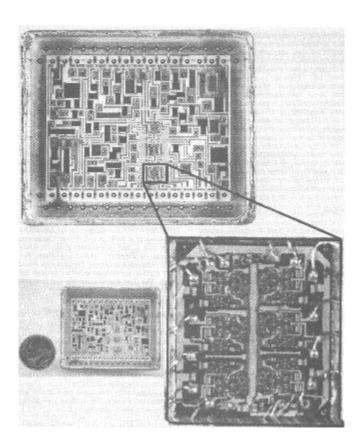
Figure 1-18.—Hybrid IC showing an enlarged chip.
