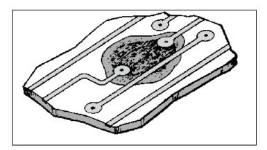
Figure 3-30.—Repaired board ready for components.
