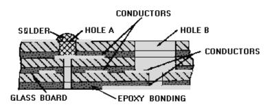
Figure 1-40.—Clearance-hole interconnection.
