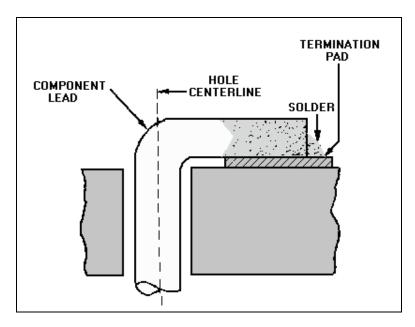
Figure 3-7A.—Offset pad termination SIDE VIEW.
