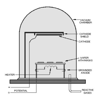
Figure 1-16.—Cathode-sputtering system.
