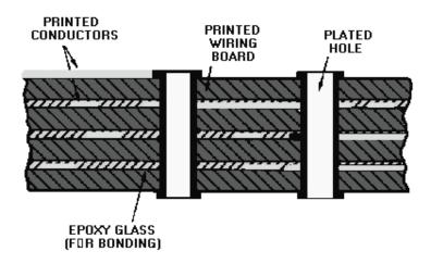
Figure 1-41.—Plated through-hole interconnection.
