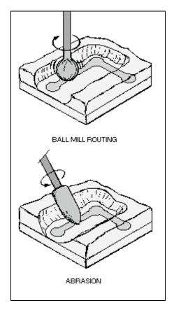
Figure 3-3.—Rotary tool conformal coating removal.
