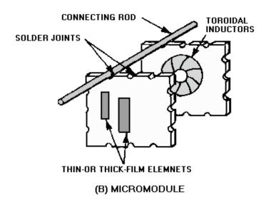
Figure 1-43B.—Evolution of modular assemblies. MICROMODULE.
