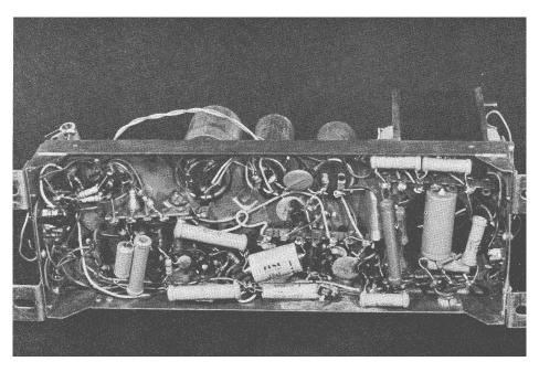
Figure 1-2.—Point-to-point wiring.
