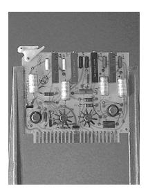
Figure 1-37.—Printed circuit board (pcb).
