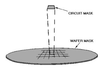
Figure 1-8.—Wafer mask distribution.
