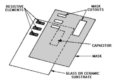
Figure 1-17.—Cathode-sputtering mask.
