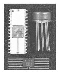
**FLIP CHIPS** and **BEAM-LEAD CHIPS** are techniques being developed to eliminate bonding wires and to improve packaging.
