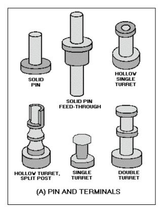
Figure 3-8A.—Terminals. PIN AND TERMINALS.
