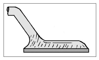
Figure 3-9.—On-the-board termination.
