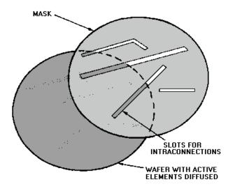
Figure 1-15.—Evaporation mask.
