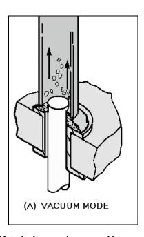
Figure 3-12A.—Motorized vacuum/pressure solder removal. VACUUM MODE.
