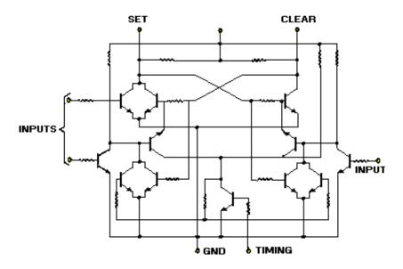
Figure 1-28.—Schematic diagram of a J-K flip-flop.
