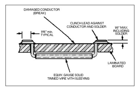
Figure 3-24.—Clinched-staple repair of broken conductor.
