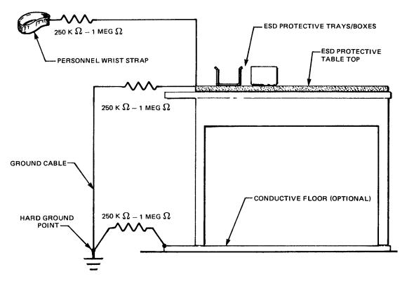
Figure 3-33.—Typical ESD ground work bench.
