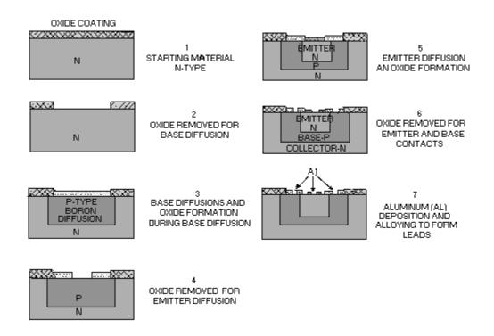
Figure 1-12.—Planar-diffused transistor.
