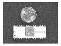
Figure 1-25.—Dual inline package (DIP).
