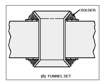
Figure 3-4B.—Eyelets (interfacial connections). FUNNEL SET
