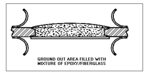
Figure 3-27.—Repair of cracked pcbs.
