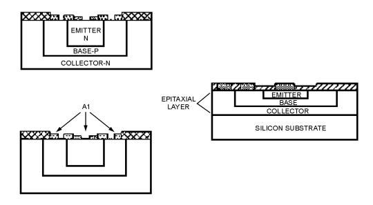
**ISOLATION** is a production method to prevent unwanted interaction between elements within a chip.
