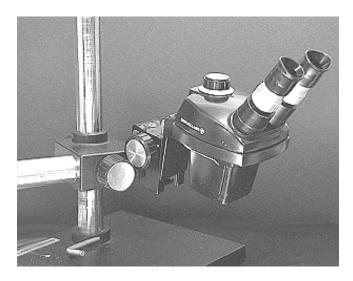
Figure 2-14.—Stereoscopic zoom microscope.
