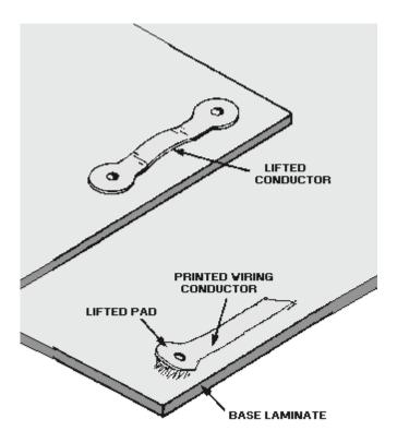
Figure 3-26.—Delaminated conductors.
