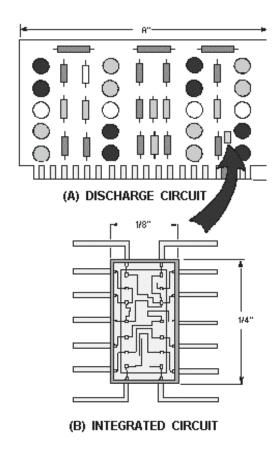
Figure 1-29.—J-K flip-flop discrete component and an IC.
