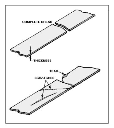
Figure 3-23.—Pcb conductor damage.
