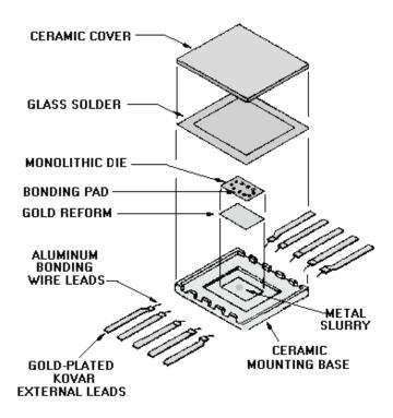
Figure 1-22.—Enlarged flat pack exploded view.
