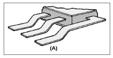
Figure 3-22A.—Properly formed flat pack leads.
