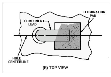
Figure 3-7B.—Offset pad termination TOP VIEW
