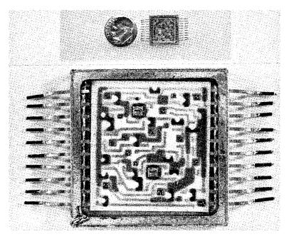
Figure 1-5.—Hybrid integrated circuit.
