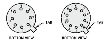
Figure 1-31.—Lead numbering for a TO-5.
