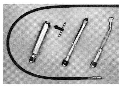
Figure 2-5.—Rotary-drive machine handpieces.
