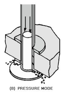
Figure 3-12B.—Motorized vacuum/pressure solder removal. PRESSURE MODE.
