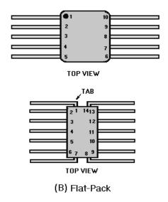
Figure 1-30B.—DIP and flat-pack lead numbering. Flat-Pack
