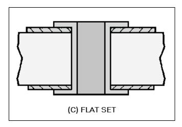
Figure 3-4C.—Eyelets (interfacial connections). FLAT SET
