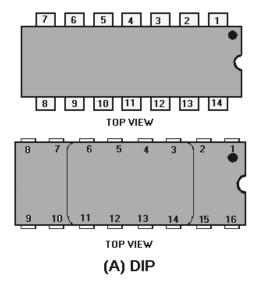
Figure 1-30A.—DIP and flat-pack lead numbering. DIP
