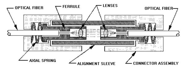
Figure 4-20.—Expanded-beam connector operation.
