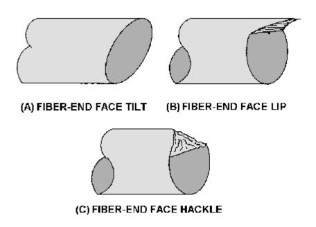
Figure 4-5.—Poor fiber-end preparation.
