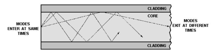
Figure 2-25.—Distance traveled by each mode over the same time span.
