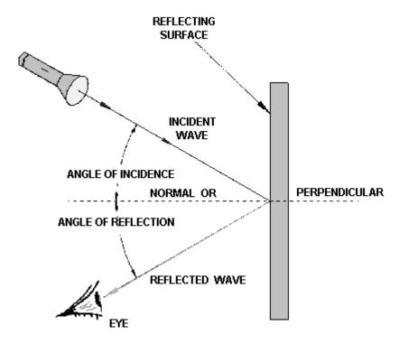
The LAW OF REFLECTION states that the angle of incidence is equal to the angle of reflection.
