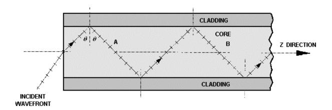
Figure 2-15.—Wavefront propagation along an optical fiber.
