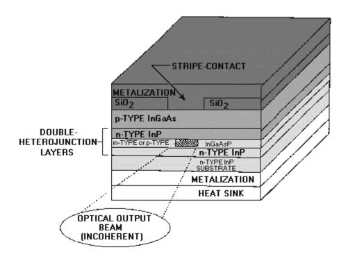
Figure 6-2.—Example of the ELED structure.
