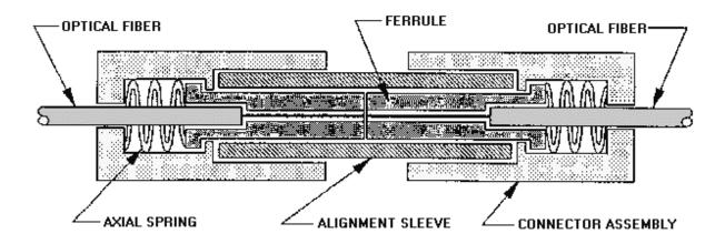
Figure 4-16.—Basic ferrule connector design.
