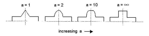
Figure 3-4.—The refractive index profiles for different values of  $\alpha$ .
