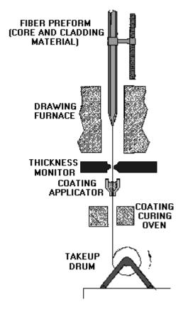
Figure 3-11.—Fiber drawing process.
