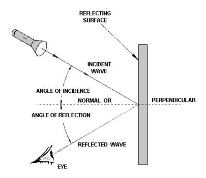
Figure 2-4.—Reflection of a wave.
