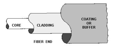
The **RAY THEORY** describes how light rays propagate along an optical fiber. **MERIDIONAL RAYS** pass through the axis of the optical fiber. **SKEW RAYS** propagate through an optical fiber without passing through its axis.
