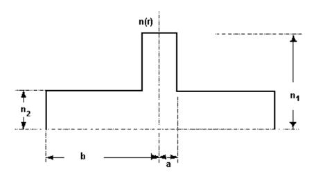
Figure 3-6.—Matched-clad refractive index profile.
