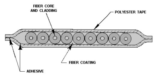
Figure 3-17.—Cross section of a fiber optic ribbon.
