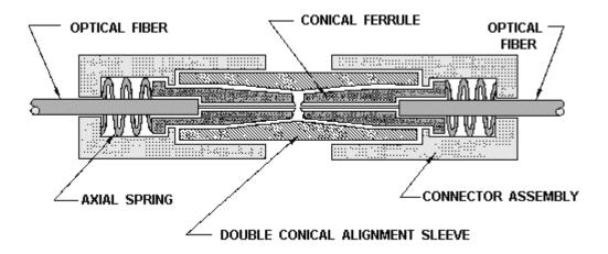
Figure 4-18.—Biconical connector design.
