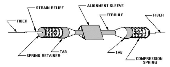
Figure 4-12.—Rotary mechanical splice.
