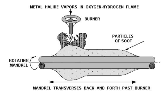
Figure 3-8.—OVPO preform preparation.
