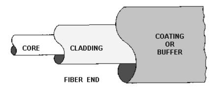
Figure 2-9.—Basic structure of an optical fiber.
