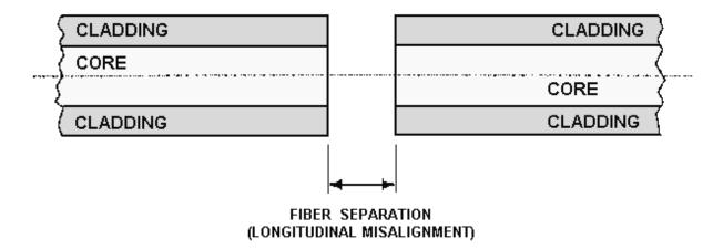
Figure 4-2.—Fiber separation.
