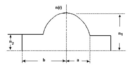
The **PROFILE PARAMETER** ( $\alpha$ ) determines the shape of the core's refractive index profile. As the value of  $\alpha$  increases, the shape of the core's profile changes from a triangular shape to a step.
