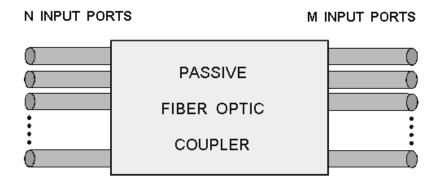
Figure 4-24.—Basic passive fiber optic coupler design.
