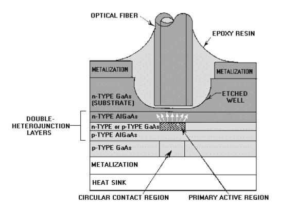
Figure 6-1.—Example of the SLED structure.
