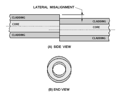
**SINGLE MODE FIBERS** are more sensitive to alignment errors than multimode fibers because of their small core diameters and low numerical apertures.
