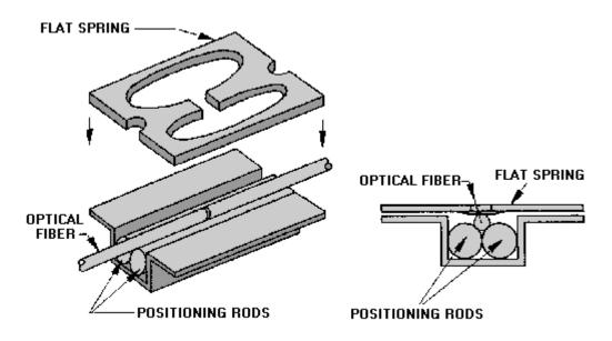
Figure 4-11.—Spring V-grooved mechanical splice.
