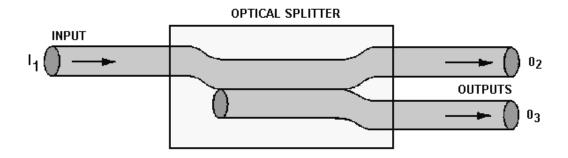
Figure 4-25.—Optical splitter.
