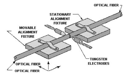
**PREFUSION** involves a short discharge of electric current across the gap between the electrodes. In prefusion the fiber ends are cleaned and rounded to eliminate any surface defects that remain from fiber cleaving.
