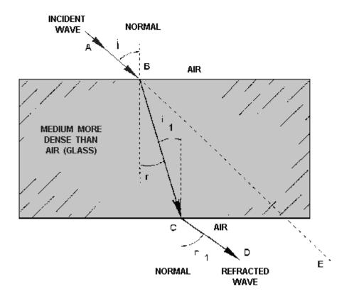
Figure 2-5.—Refraction of a wave.
