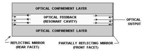
Figure 6-3.—Optical cavity for producing lasing.
