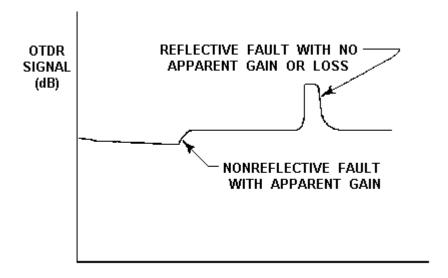
Figure 5-15.—An OTDR trace showing a nonreflective fault with apparent gain and a reflective fault with no apparent loss or gain.
