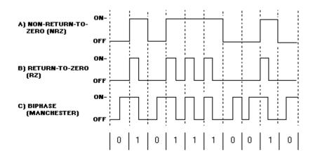
Figure 8-6.—NRZ, RZ, and biphase (Manchester) encoding.
