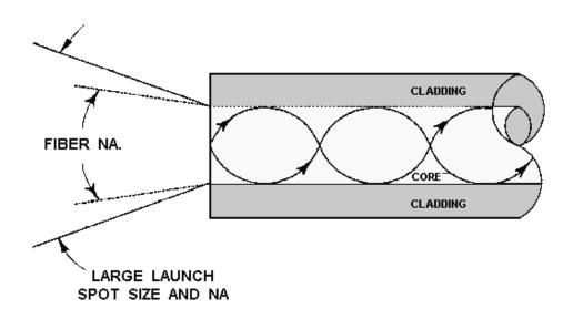
Figure 5-3.—Overfilled launch condition.
