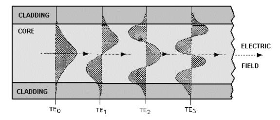
Figure 2-17.—Transverse electric (TE) mode field patterns.
