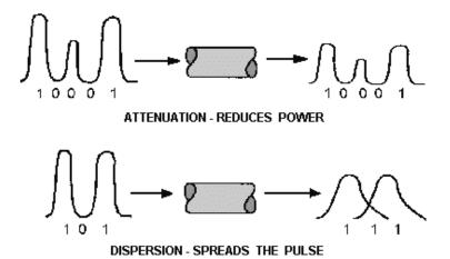
Figure 2-19.—Fiber transmission properties.
