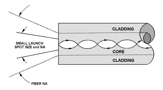
Figure 5-2.—Underfilled launch condition.
