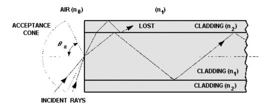
Figure 2-12.—Fiber acceptance angle.
