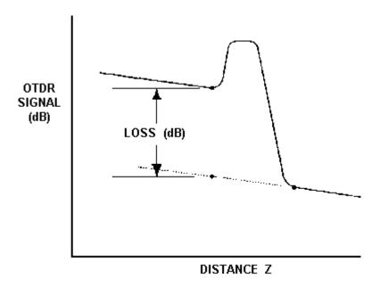
Figure 5-17.—The exaggerated loss obtained at point defects exhibiting gain in one direction by conducting the OTDR measurement in the opposite direction.
