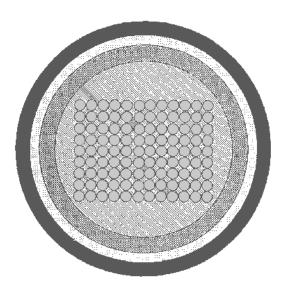
Figure 3-18.—Ribbon cable cross-sectional array of fibers.
