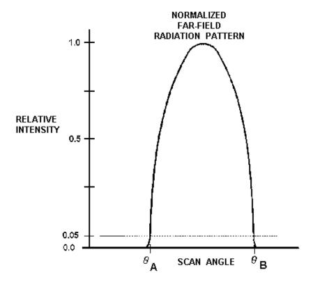
Figure 5-11.—Normalized far-field radiation pattern.
