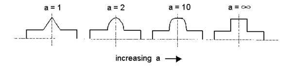
The gradual decrease in the core's refractive index from the center of the fiber causes propagating modes to be refracted many times.
