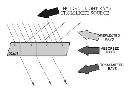
**REFLECTION** occurs when a wave strikes an object and bounces back (toward the source). The wave that moves from the source to the object is called the **incident wave**, and the wave that moves away from the object is called the **reflected wave**.
