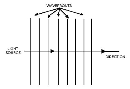
Figure 2-14.—Plane-wave propagation.
