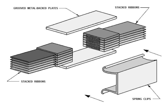
Figure 4-19.—Spring clip method of ribbon connection.
