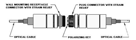
Figure 4-22.—MIL-C-28876 heavy-duty connector.
