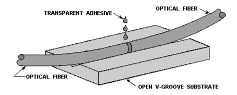
Figure 4-10.—Open V-grooved splice.
