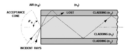
**NUMERICAL APERTURE (NA)** is a measurement of the ability of an optical fiber to capture light.
