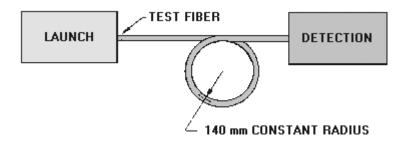
Figure 5-5.—Single-turn configuration for the test fiber.
