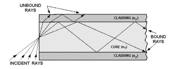
The **ACCEPTANCE ANGLE** is the maximum angle to the axis of the fiber that light entering the fiber is bound or propagated. The light ray incident on the fiber core must be within the acceptance cone defined by the acceptance angle to be propagated along an optical fiber.
