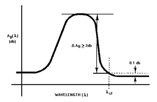
Figure 5-6.—Fiber cutoff wavelength determined by the bend-reference technique.
