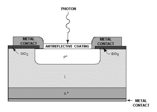
Figure 7-2.—The basic structure of a PIN photodiode.
