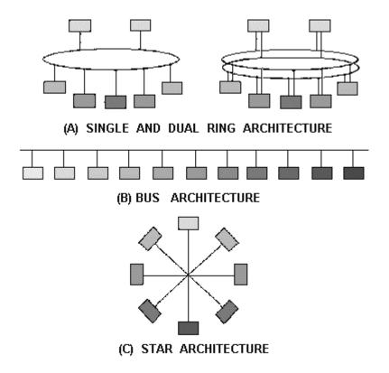
Figure 4-23.—Examples of complex system architectures.
