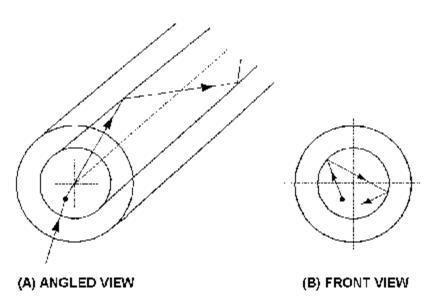
Figure 2-13.—Skew ray propagation: A. Angled view; B. Front view.
