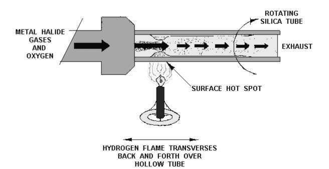
Figure 3-9.—IVPO preform preparation.
