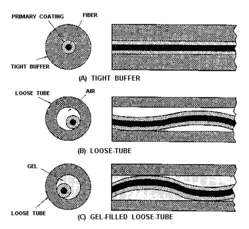
Figure 3-13.—Tight-buffered, loose-tube, and gel-filled loose-tube buffer techniques.
