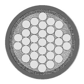
Figure 3-16.—Stranded cable design.
