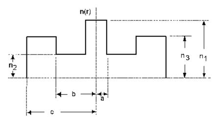
Figure 3-7.—Depressed-clad refractive index profile.
