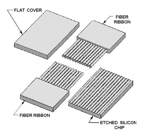
Figure 4-14.—Ribbon splice on etched silicon chip.
