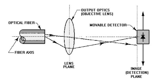
Figure 5-8.—The measurement of the near-field power distribution.
