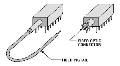
Figure 4-1.—Pigtailed and connectorized fiber optic devices.
