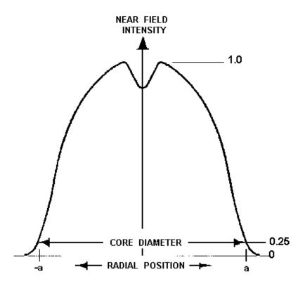
Figure 5-9.—Near-field radiation pattern.
