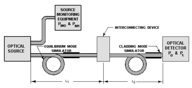
Figure 5-12.—Insertion loss measurement of an interconnecting device.
