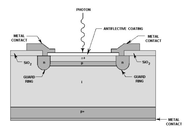
Figure 7-4.—The basic structure of an APD.
