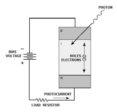
Figure 7-3.—A schematic representation of a photodiode.
