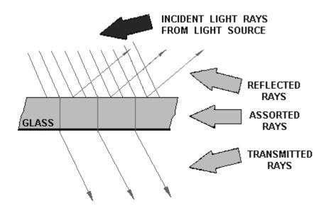
Figure 2-2.—Light waves reflected, absorbed, and transmitted.
