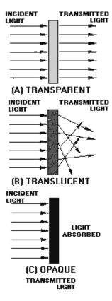
Figure 2-3.—Substances: A. Transparent; B. Translucent; and C. Opaque.
