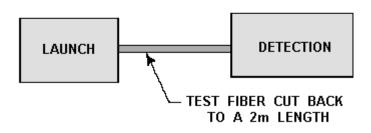
Figure 5-1.—Cutback method for measuring fiber attenuation: A. Test measurement; B. Cut-back measurement.
