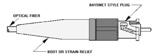
Figure 4-21.—ST light-duty connector.
