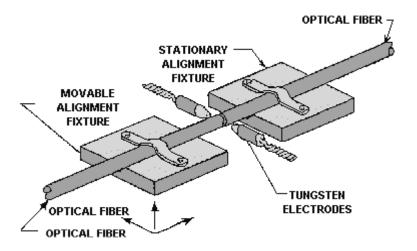
Figure 4-13.—A basic fusion splicing apparatus.
