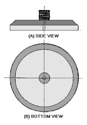
Figure 4-7.—Fiber polishing tool.
