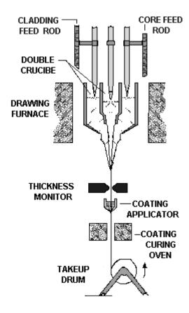
Figure 3-12.—Double-crucible fiber drawing process.
