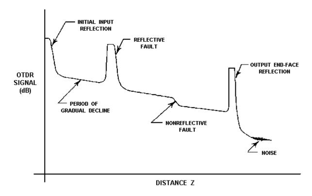
Figure 5-13.—OTDR trace of an installed cable plant.
