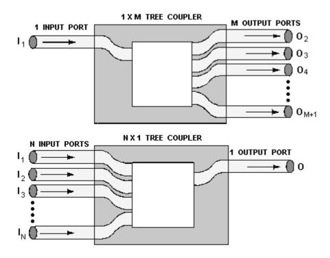
Figure 4-28.— $(1 \times M)$  and  $(N \times 1)$  tree coupler designs.
