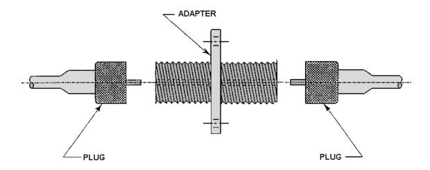
Figure 4-15.—Plug-adapter-plug configuration.
