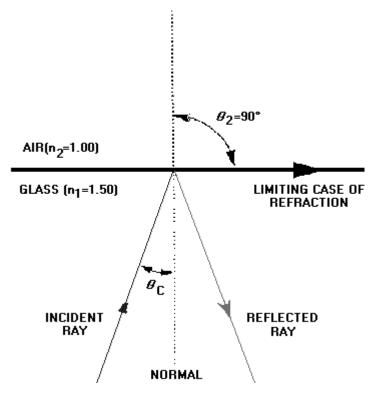
Figure 2-8.—Critical angle of incidence.
