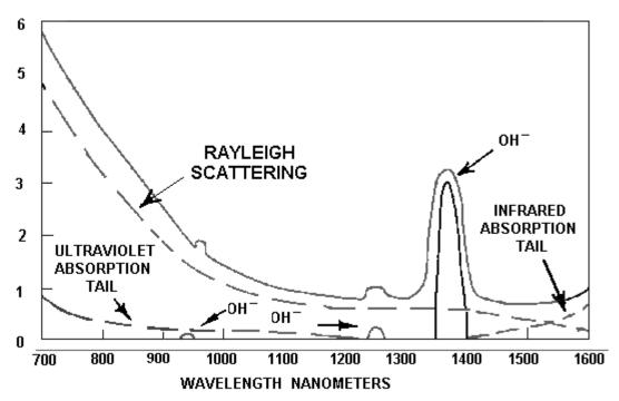
**SCATTERING** losses are caused by the interaction of light with density fluctuations within a fiber. **Rayleigh scattering** is the main source of loss in commercial fibers operating between 700 nm and 1600 nm.
