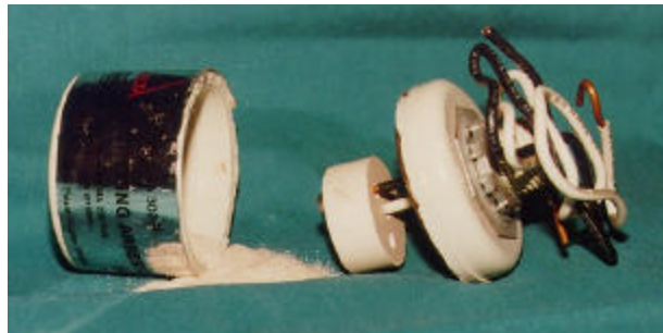
Figure D-2. Unlisted Surge Protector
