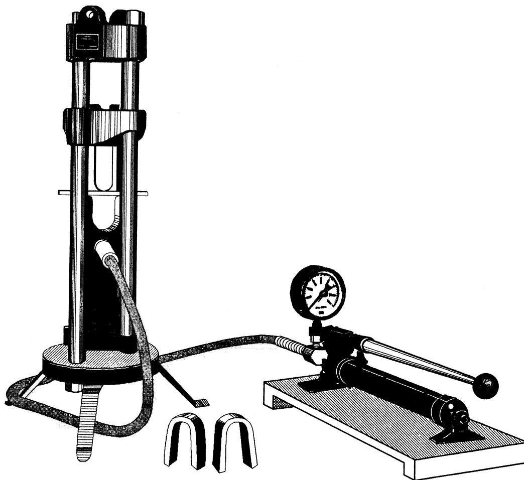
Figure 7-64.—Testing machine for making guided-bend tests.
