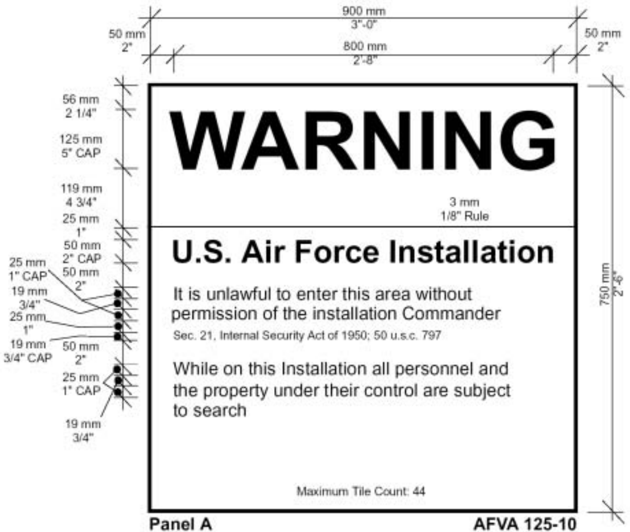
Figure 6.5. Base Warning Sign Type E1 Panel A.
