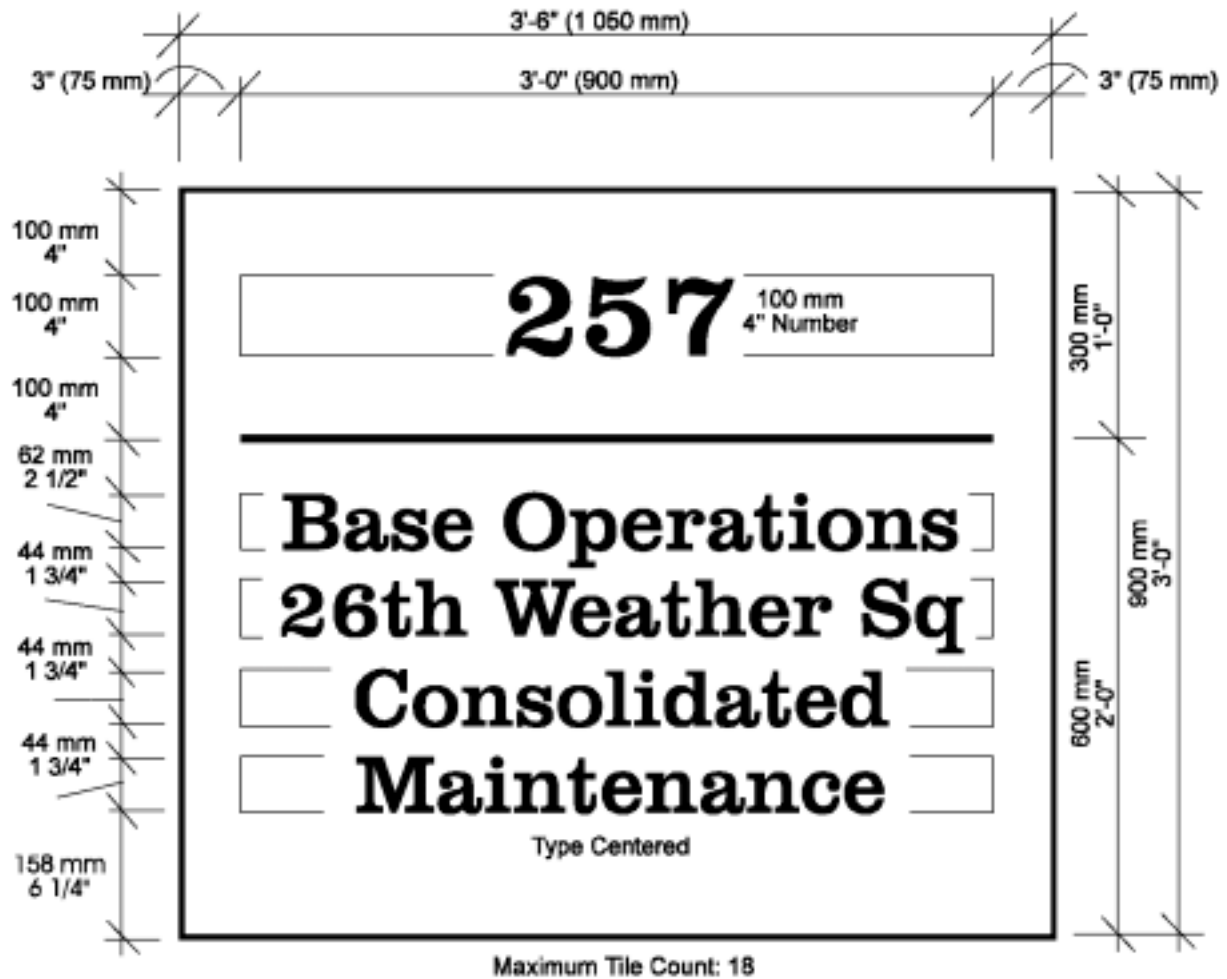
Figure 9.6. Building Identification Sign Type H1 Expanded Layout.
