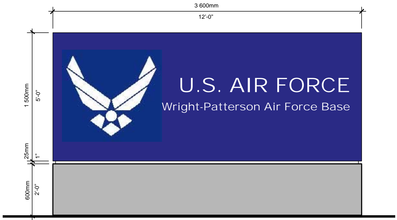
Figure 4.4. Main Entrance Sign Type A1 Dimensions.
