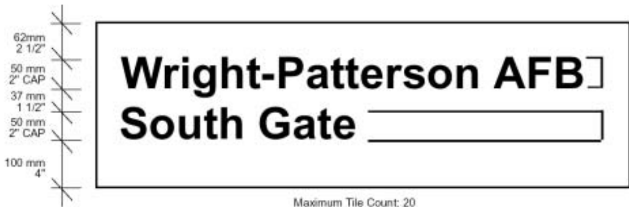
Figure 4.10. Entry Gate Type A3 Expanded Layout.
