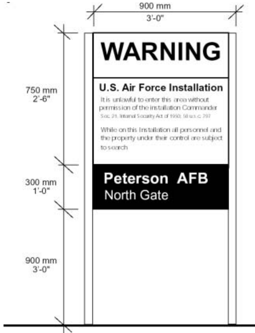
Figure 4.8. Entry Gate Sign Type A3 Dimensions.
