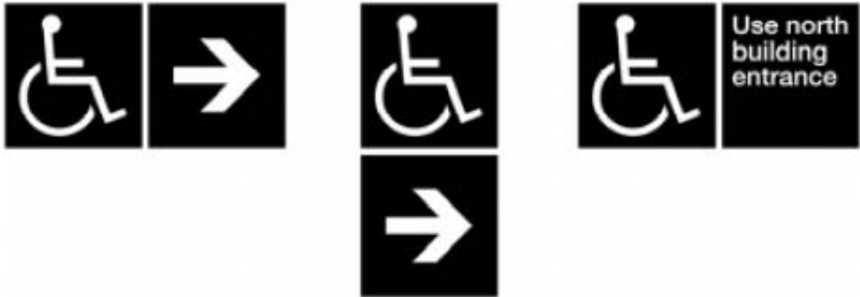
Figure 5.12. Direction Sign Type D3, Typical Configurations.
