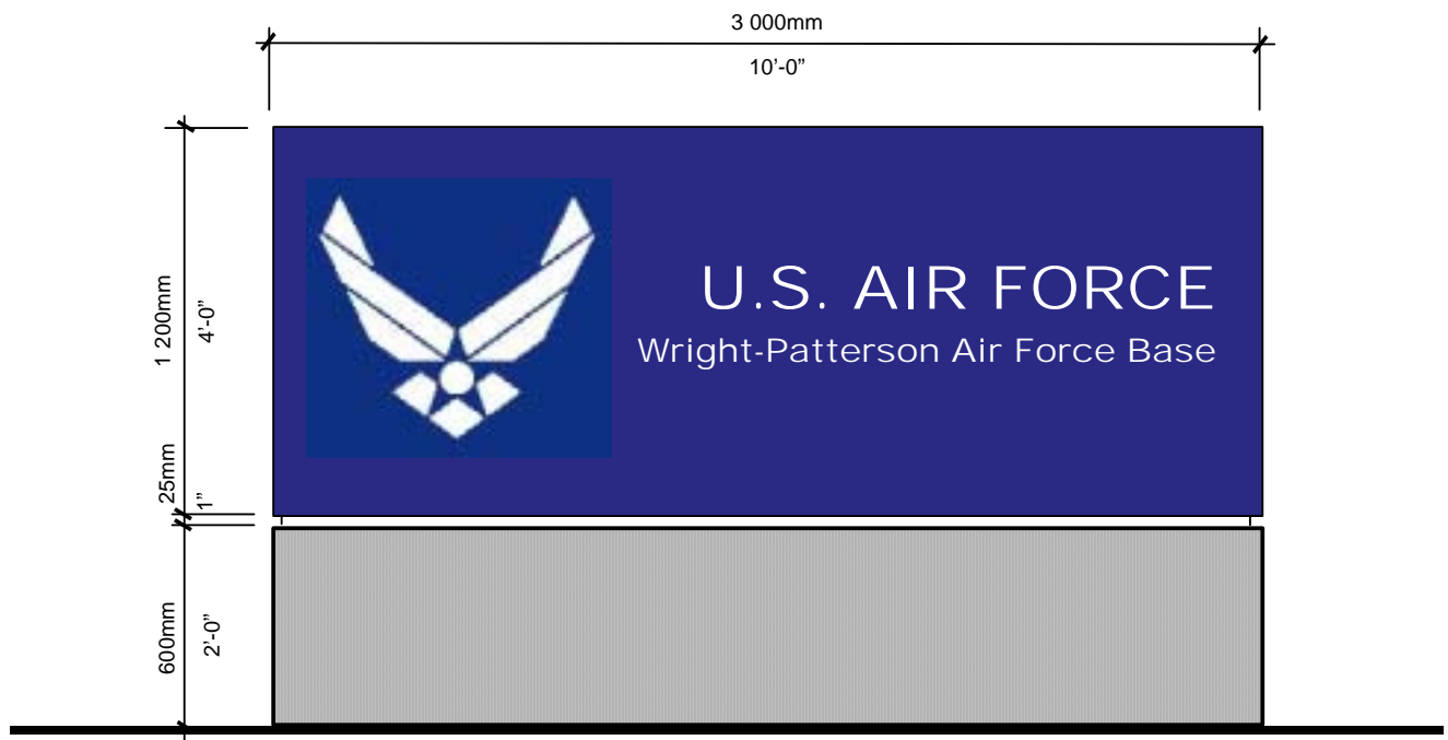
Figure 4.6. Secondary Entrance Sign Type A2 Dimensions.
