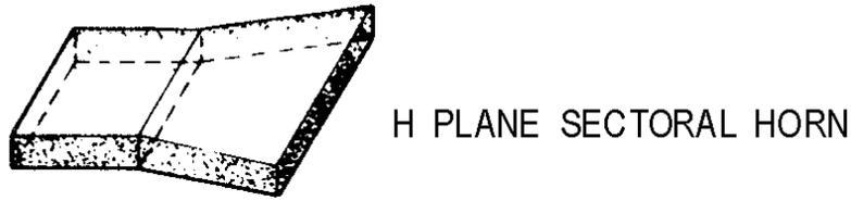
Figure 1-44B.—Waveguide horns. H PLANE SECTORAL HORN.
