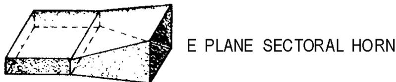
Figure 1-44A.—Waveguide horns. E PLANE SECTORAL HORN.
