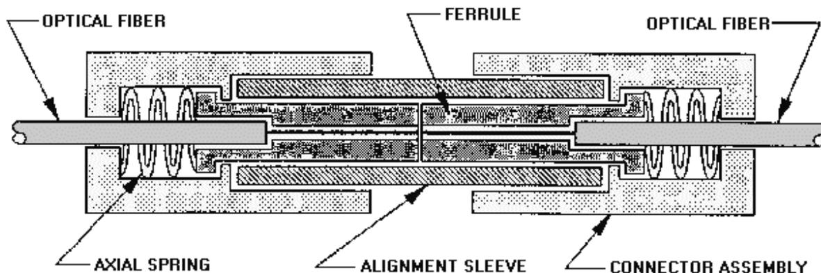
Figure 4-16.—Basic ferrule connector design.
