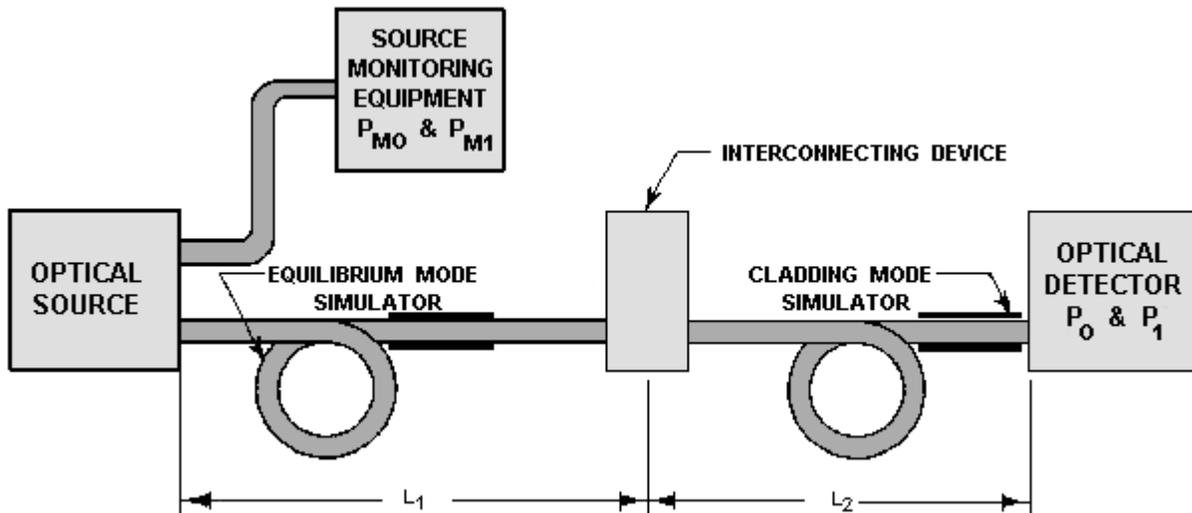
Figure 5-12.—Insertion loss measurement of an interconnecting device.
