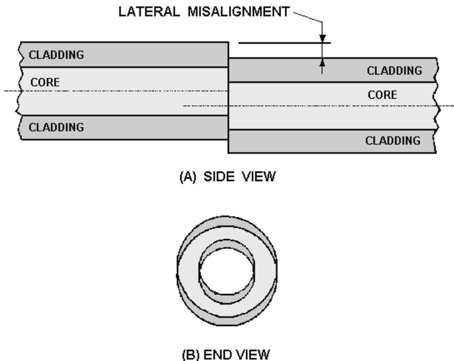
**SINGLE MODE FIBERS** are more sensitive to alignment errors than multimode fibers because of their small core diameters and low numerical apertures.
