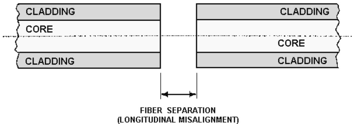
Figure 4-2.—Fiber separation.
