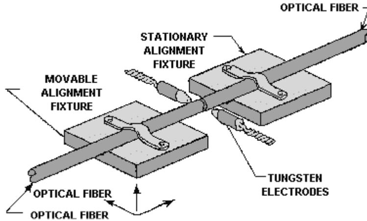
**PREFUSION** involves a short discharge of electric current across the gap between the electrodes. In prefusion the fiber ends are cleaned and rounded to eliminate any surface defects that remain from fiber cleaving.
