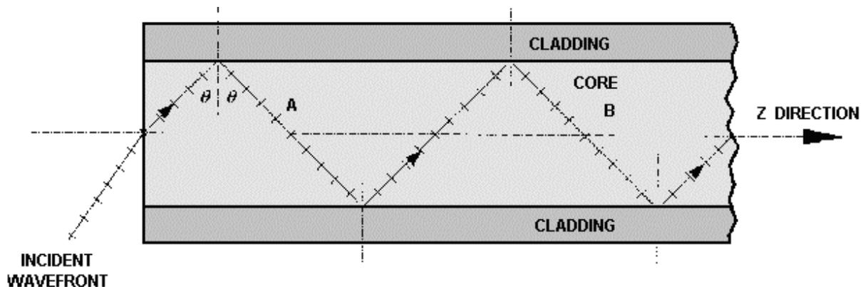
Figure 2-15.—Wavefront propagation along an optical fiber.
