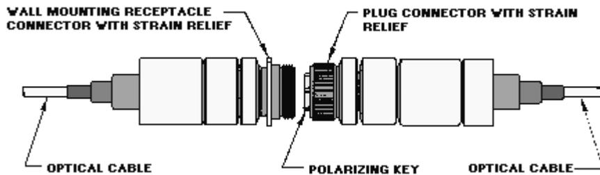
Figure 4-22.—MIL-C-28876 heavy-duty connector.
