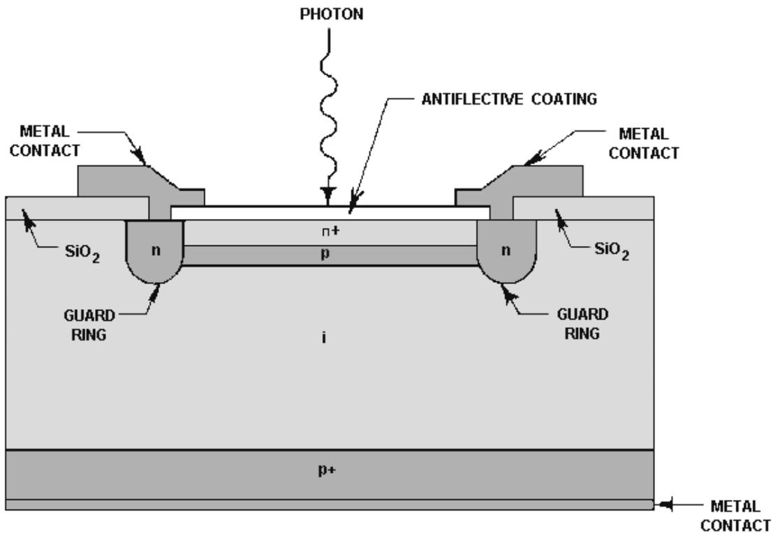
Figure 7-4.—The basic structure of an APD.
