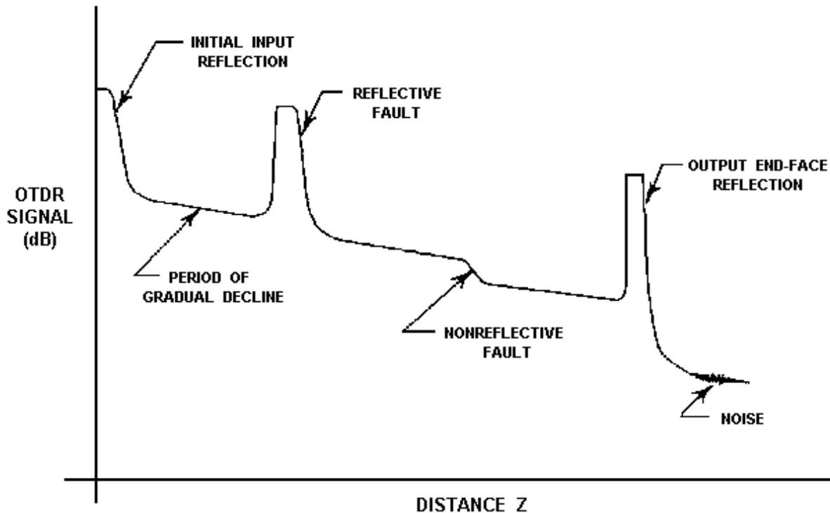
Figure 5-13.—OTDR trace of an installed cable plant.
