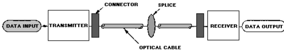
Figure 1-1.—Parts of a fiber optic data link.
