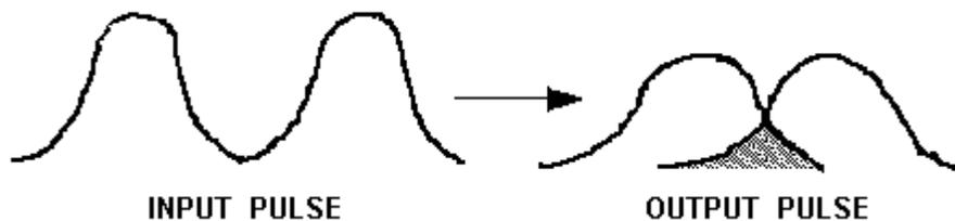
Figure 2-16.—The spreading of a light pulse.
