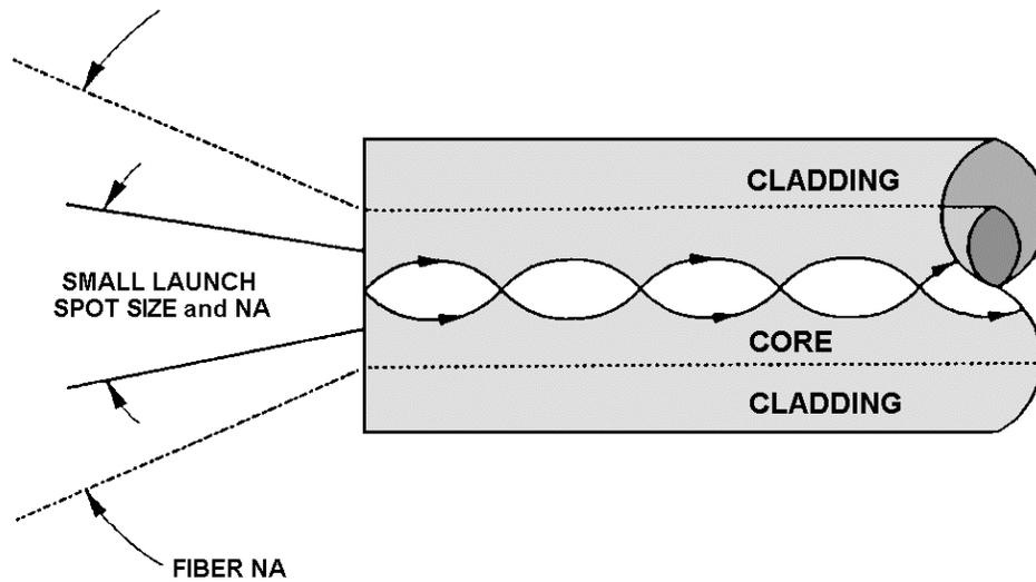
Figure 5-2.—Underfilled launch condition.
