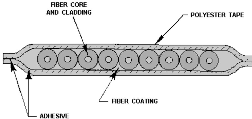
Figure 3-17.—Cross section of a fiber optic ribbon.
