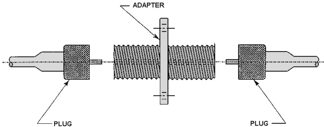
Figure 4-15.—Plug-adapter-plug configuration.
