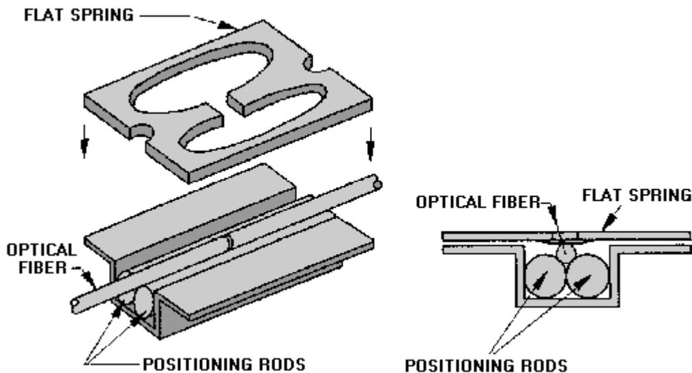
Figure 4-11.—Spring V-grooved mechanical splice.
