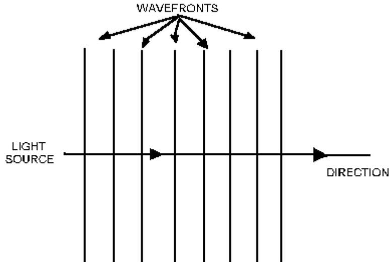
Figure 2-14.—Plane-wave propagation.
