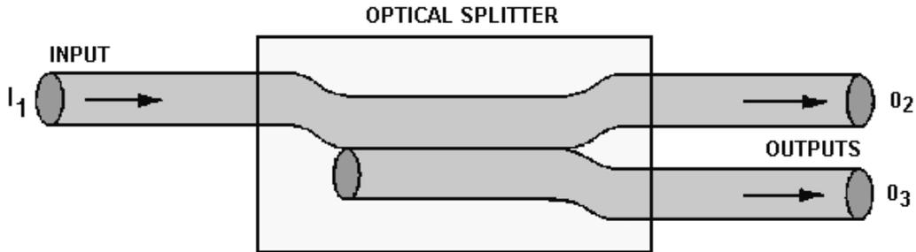
Figure 4-25.—Optical splitter.
