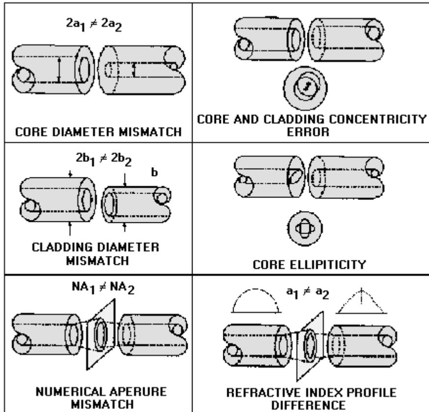
**CORE DIAMETER MISMATCH** causes coupling loss only if the launching fiber has a larger core radius than the receiving fiber.
