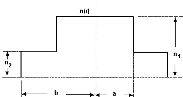
The **RELATIVE REFRACTIVE INDEX DIFFERENCE ( $\Delta$ )** is the difference in the core and cladding refractive index. The ability of the fiber to accept optical energy from a light source is related to  $\Delta$ .
