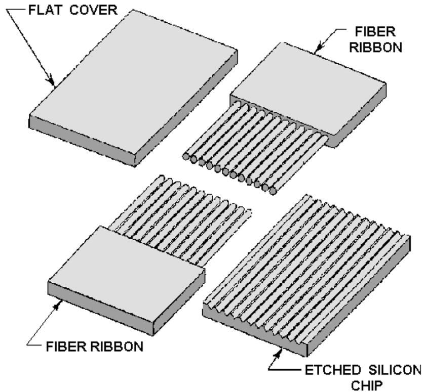
Figure 4-14.—Ribbon splice on etched silicon chip.
