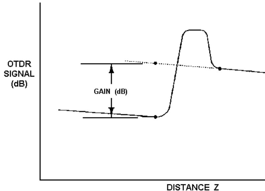
Figure 5-16.—Extrapolation for a point defect showing an apparent signal gain.
