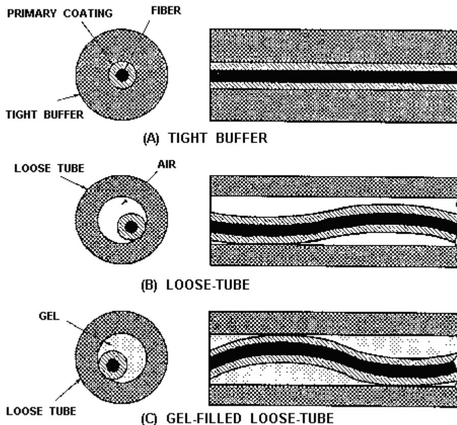
Figure 3-13.—Tight-buffered, loose-tube, and gel-filled loose-tube buffer techniques.
