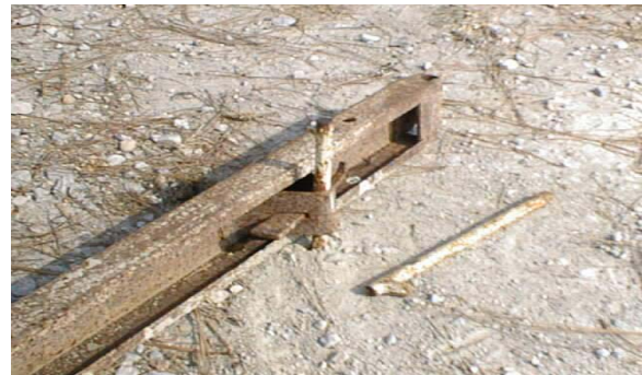
Figure 3-2. Metal Stake And Wedge For Form.
