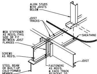
**JOIST SUPPORTED BY BEAM (ALTERNATE)**
