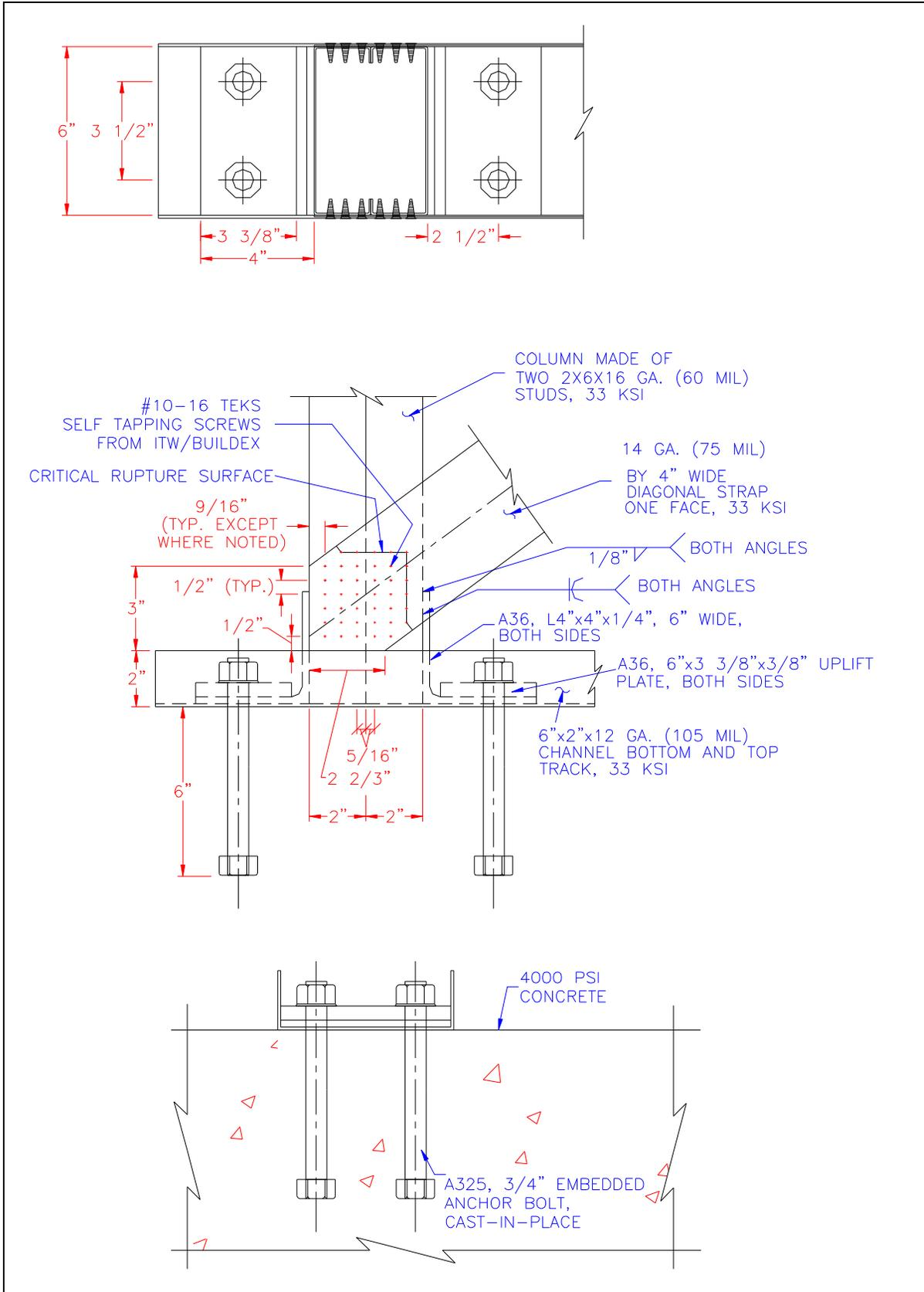
Figure D-4. Example connection/anchorage detail – 1<sup>st</sup> row of Tables D-5, D-8 – D-17.
