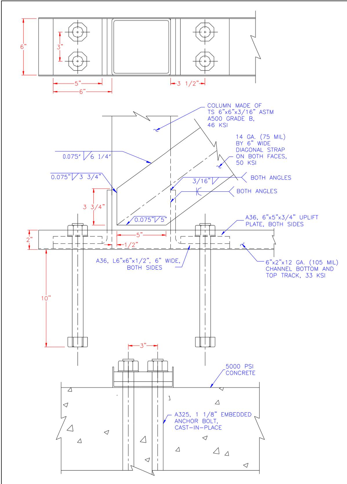
Figure D-9. Example connection/anchorage detail - 6<sup>th</sup> row of Tables D-5, D-8 - D-17.
