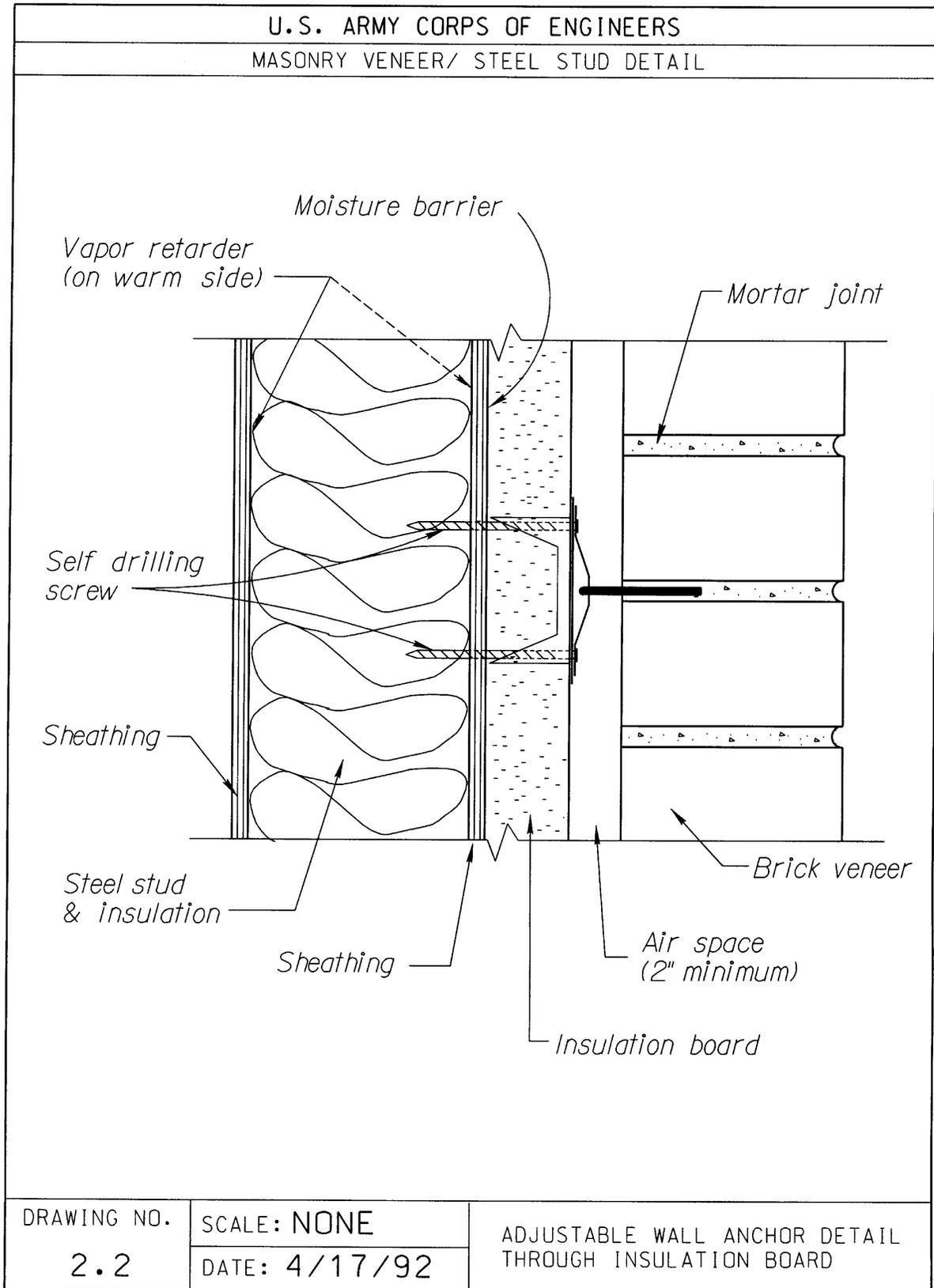
Figure G-6. Adjustable Wall Anchor Detail
