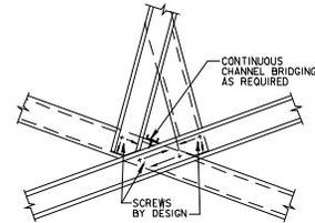
**BOTTOM CHORD INTERSECTION ON SCISSORS TRUSS**
