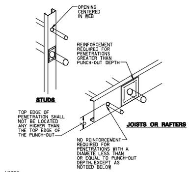
**JOIST STUD OR RAFTER WEB PENETRATIONS**
