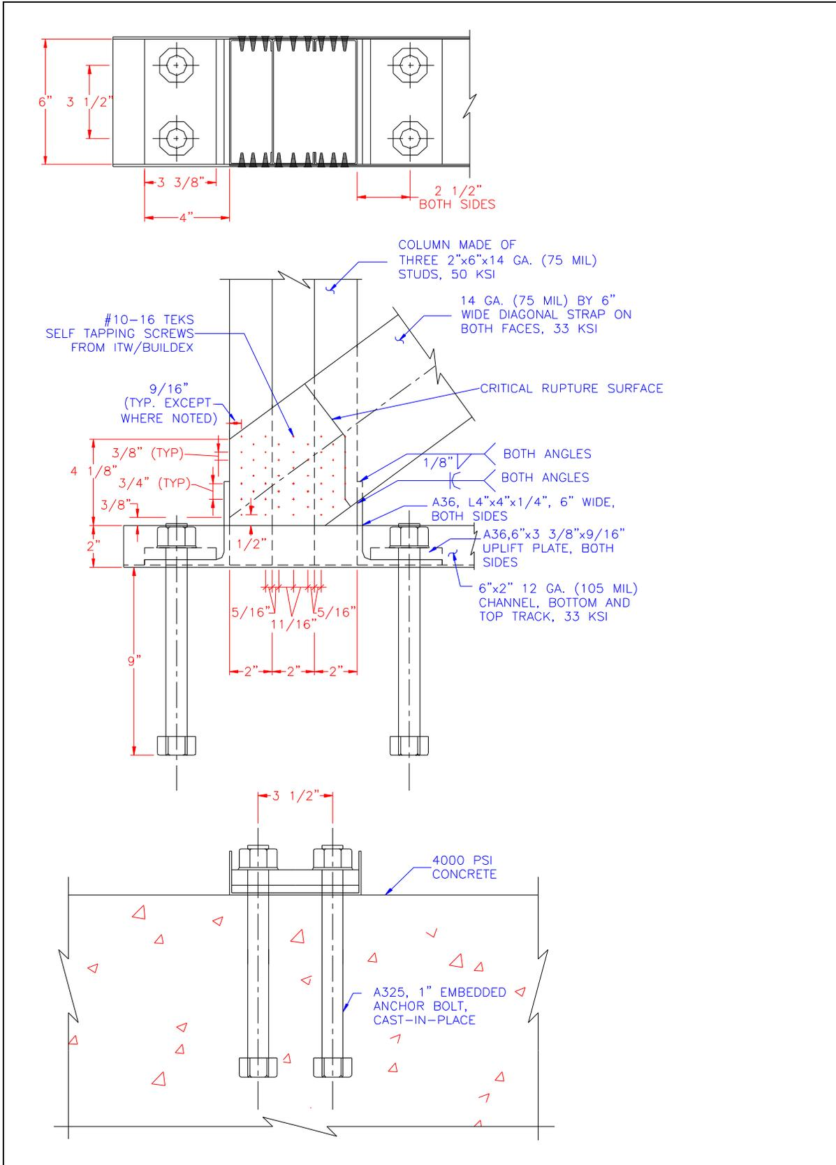
Figure D-6. Example connection/anchorage detail – 3<sup>rd</sup> row of Tables D-5, D-8 - D.17.
