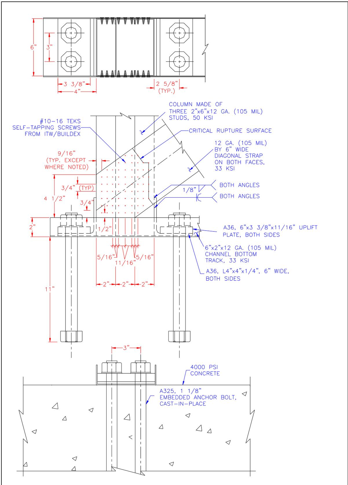
Figure D-7. Example connection/anchorage detail - 4<sup>th</sup> row of Tables D-5, D-8 – D-17.
