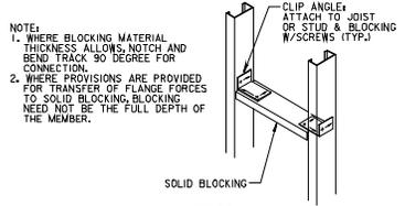
**JOISTS OR RAFTERS SOLID BLOCKING**
