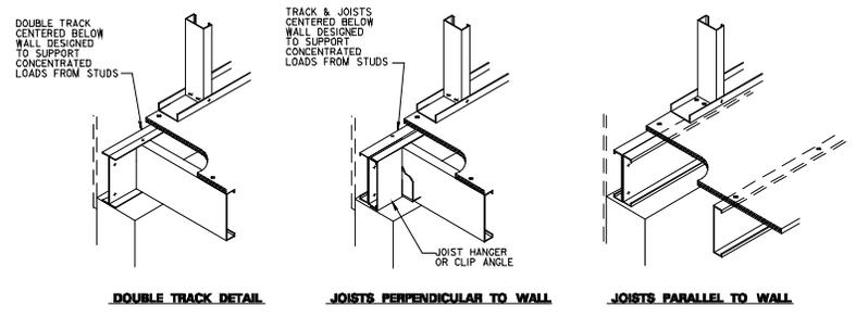
**ALTERNATE RIBBON JOIST DETAILS** (A.7H) (S.15)
