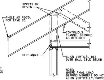
**ROOF TRUSS BEARING** (A.7B) (S.15)
