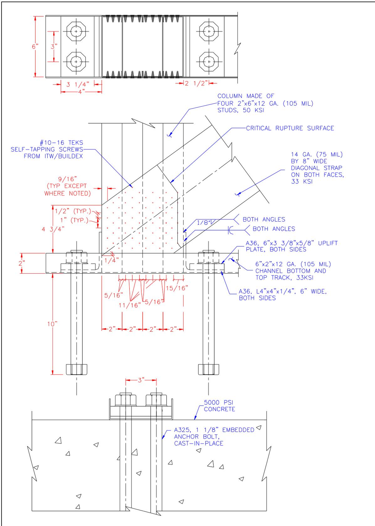
Figure D-8. Example connection/anchorage detail – 5<sup>th</sup> row of Tables D-5, D-8 – D-17.
