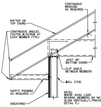
**ROOF EAVE AND SOFFIT** (A.7) (S.15)
