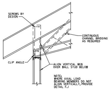
**ROOF SCISSORS TRUSS BEARING** (A.7C) (S.15)
