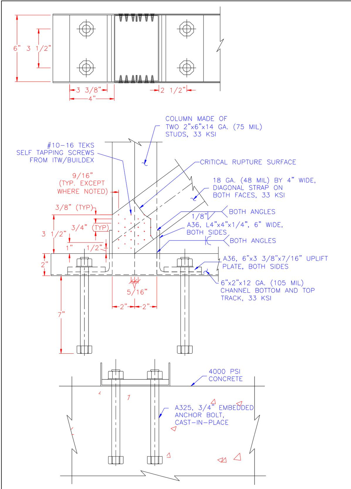
Figure D-5. Example connection/anchorage detail – 2<sup>nd</sup> row of Tables D-5, D-8 - D-17.
