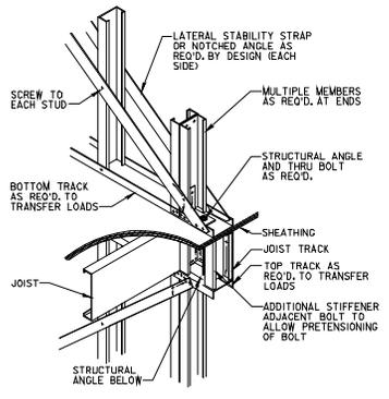
**DIAGONAL STABILITY BRACING AT FLOOR TRANSITION**
