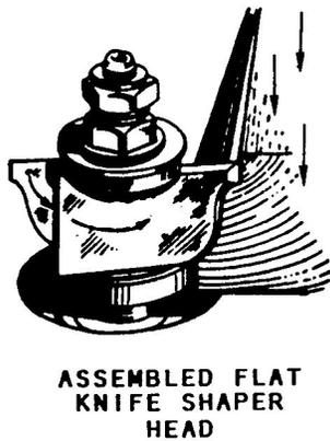
Figure 3-12.—Three-wing cutter for a shaper.
