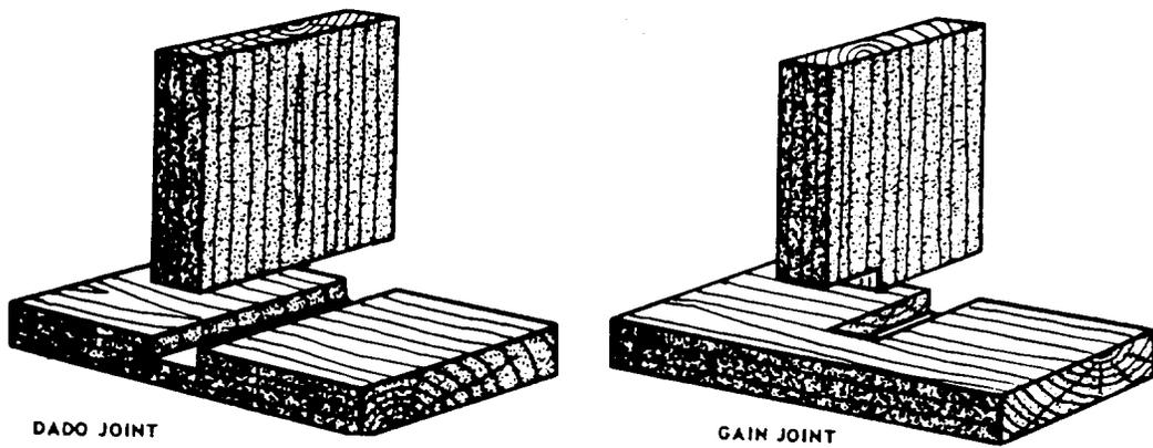
Figure 3-46.-Dado and gain joints.
