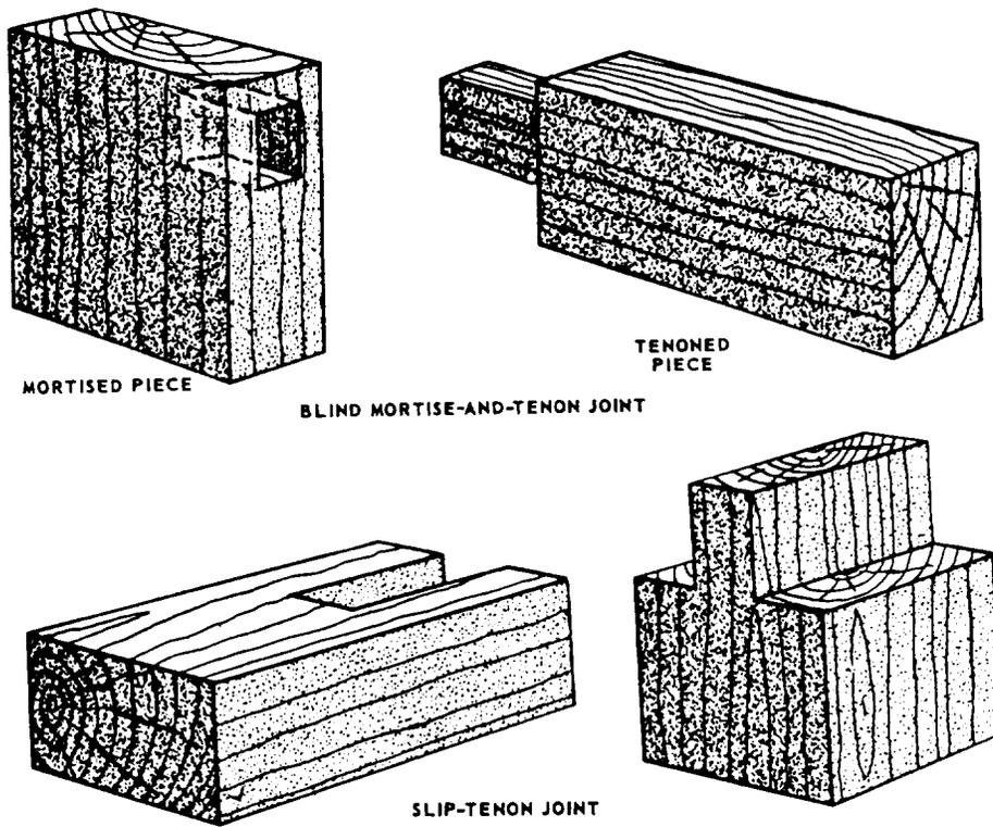
Figure 3-47.-Tenon joints.
