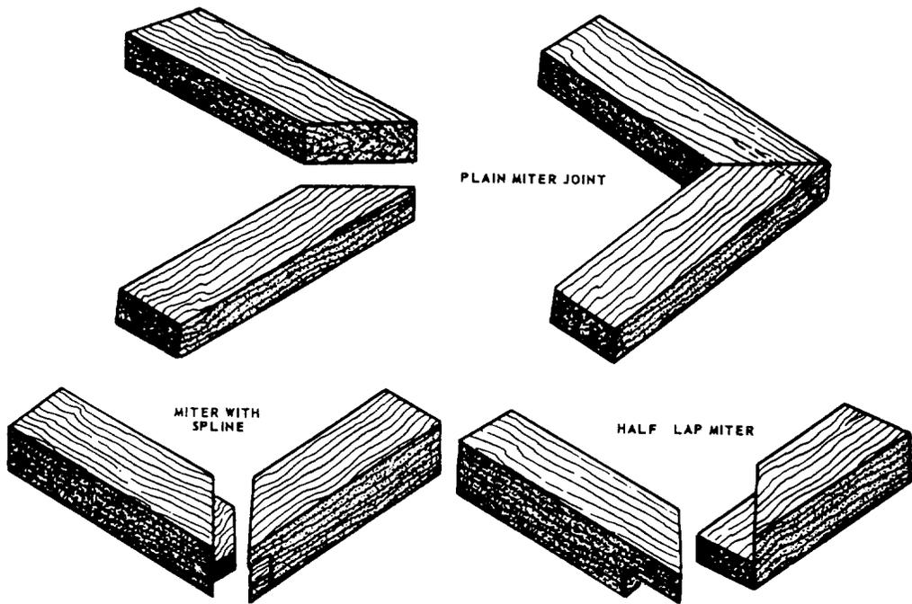
Figure 3-44.-Miter joints.
