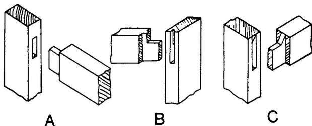
**Figure 3-55.-Stub (view A), haunched (view B), and table-haunched (view C) mortise-and-tenon joints.**
