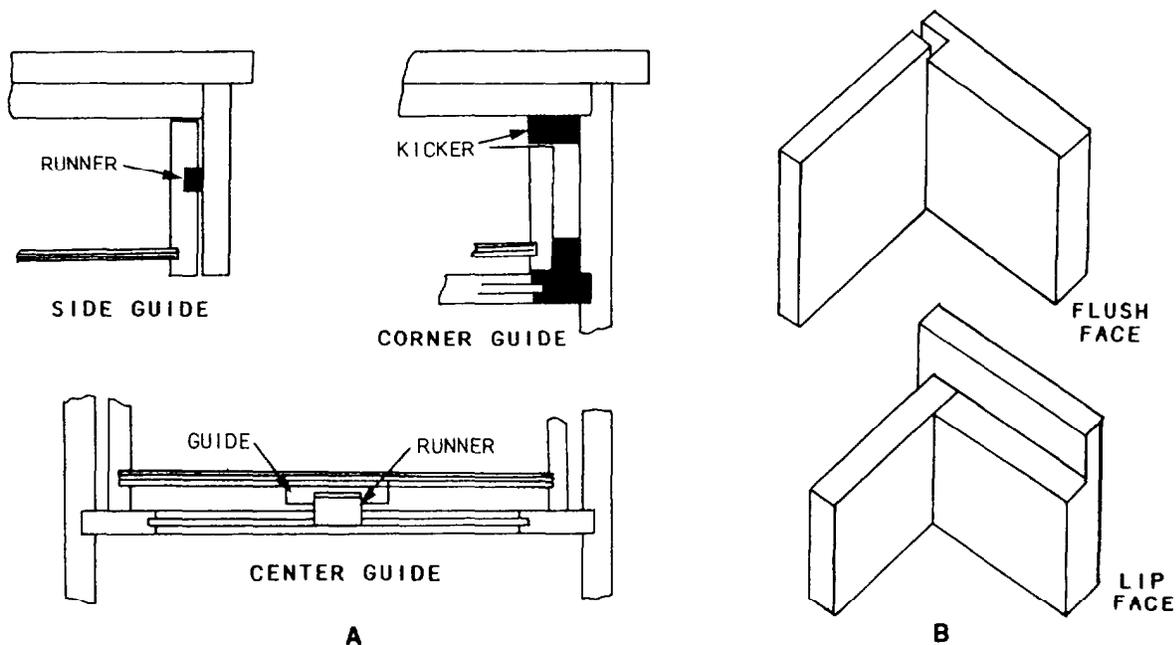
Figure 3-74.-Types of drawer guides (view A) and faces (view B).
