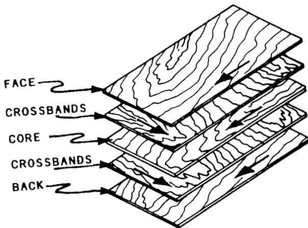
Figure 3-36.-Grain direction in a sheet of plywood.
