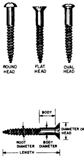
Figure 3-81.-Types and nomenclature of wood screws.
