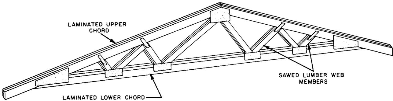
Figure 3-31.-Truss using laminated and sawed lumber.
