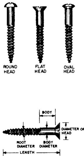
Figure 3-81.-Types and nomenclature of wood screws.
