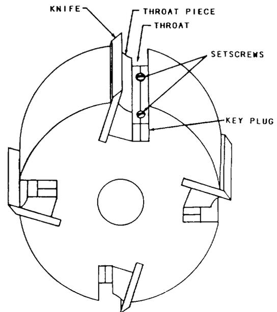
Figure 3-8.—Four-knife butterhead for a jointer.
