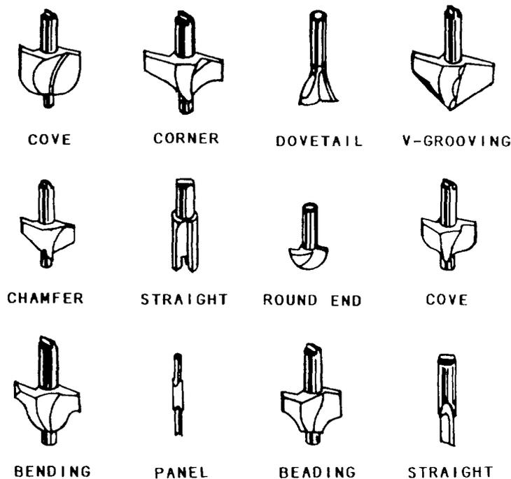
Figure 3-22.-Router bits.
