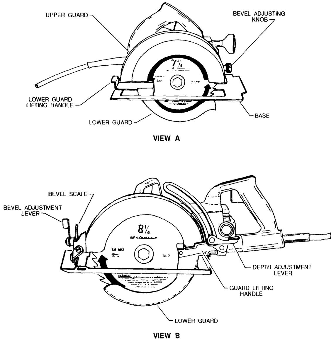
Figure 3-15.-Side-drive (view A) and worm-drive (view B) circular saws
