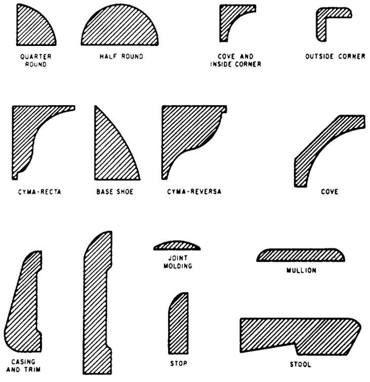
Figure 3-66.-Simple molding and trim shapes.
