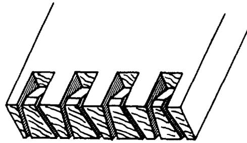
Figure 3-64.-Chiseling out waste in a through-multiple-dovetail joint.
