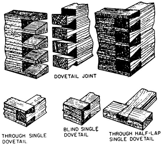
Figure 3-49.-Dovetail joints.
