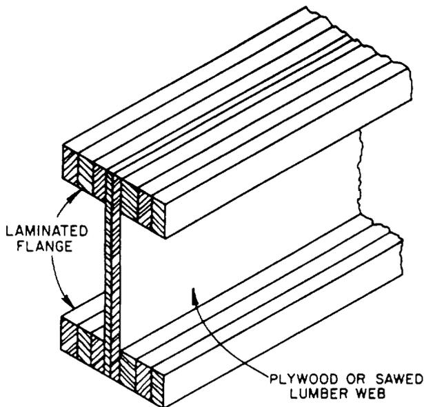
Figure 3-32.-Laminated and sawed lumber or plywood beam.
