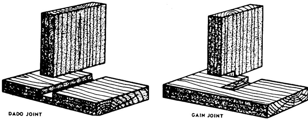
Figure 3-46.-Dado and gain joints.
