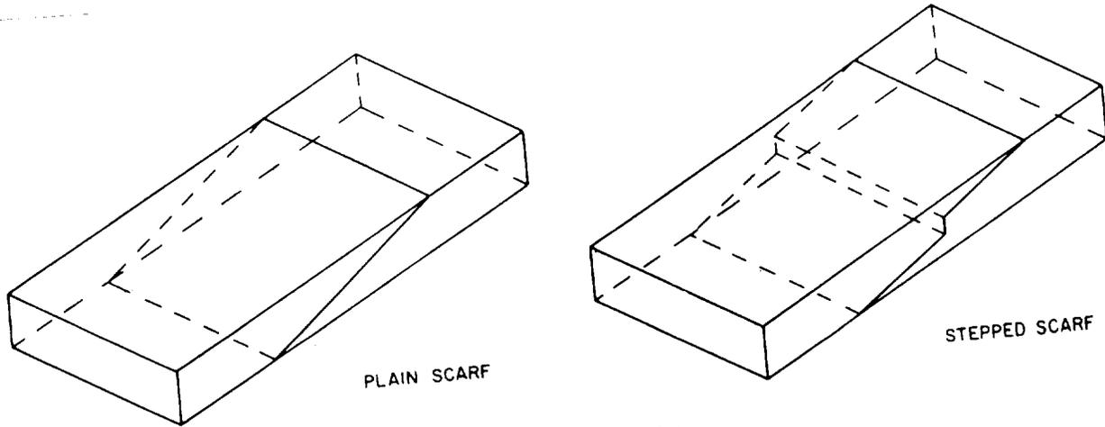
Figure 3-34.-Scarf joints.
