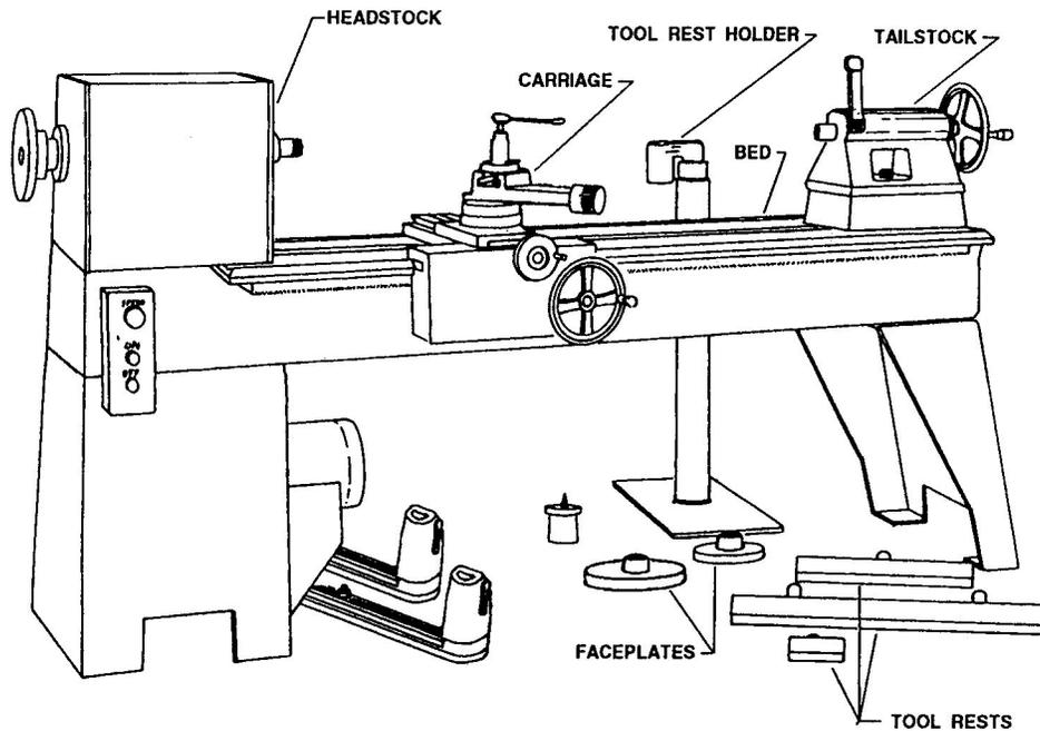
**Figure 3-5.—A woodturning lathe with accessories.**
