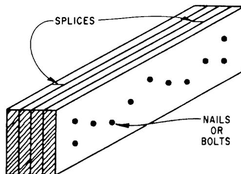
Figure 3-30.-Built-up beam.
