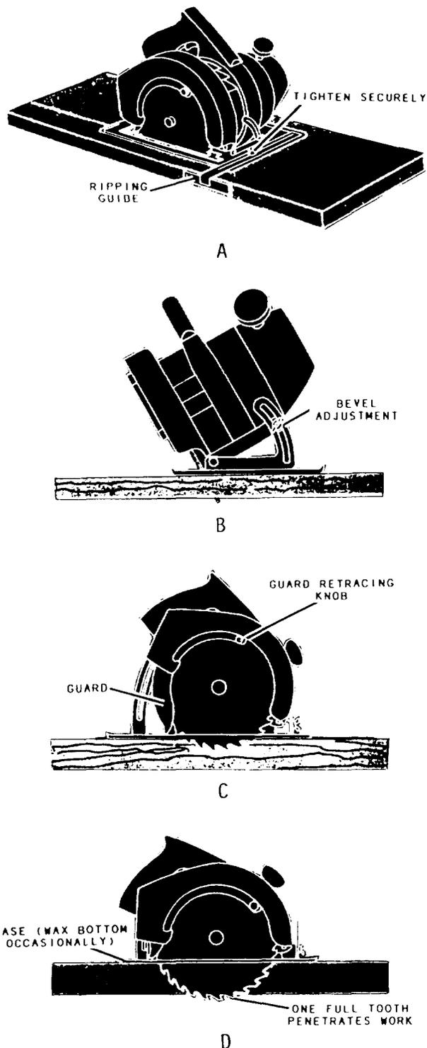
Figure 3-17.-Different ways to use a circular saw.
