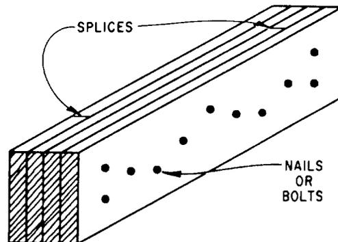
Figure 3-30.-Built-up beam.
